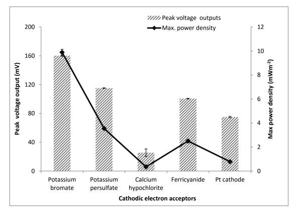
**Figure 4.7:** The electrochemical performance of the MFC using different electron acceptors at the cathode (Ext. resistance,  $R=1 \text{ k}\Omega$ ). Values are means of duplicate experiments  $\pm$  SD.
