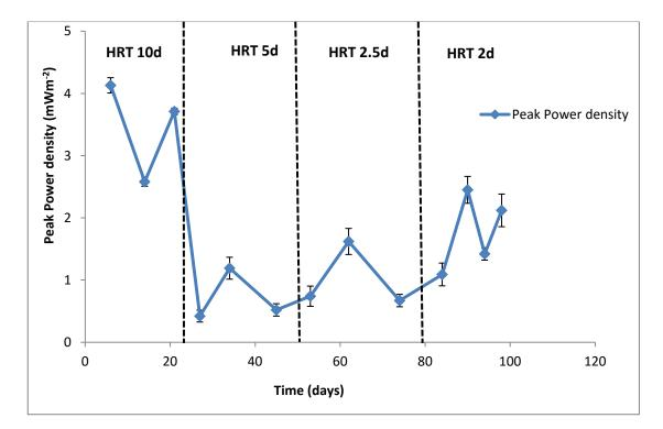
**Figure 5.2:** Profile of peak power densities produced at different HRTs in a tubular MFC over 100 days continuous operation at ambient temperatures (10-25 °C) using adapted microbial consortia. Values are means of duplicate experiments  $\pm$  SD.
