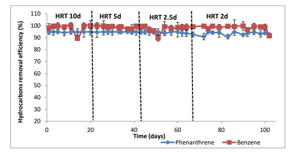
**Figure 5.1:** (A) COD removal and (B) Hydrocarbons removal efficiencies at various HRT regimes over a period of 110 days of continuous MFC operation at ambient temperatures (14-25 °C) using adapted microbial consortia. Values are means of duplicate experiments  $\pm$  SD.
