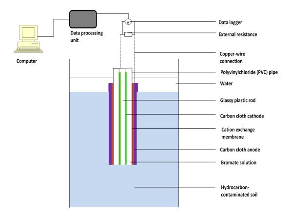
**Figure 2.4:** The schematic diagram of the tubular soil MFC reactor experimental set up employed for treating a model PAH-contaminated soil.
