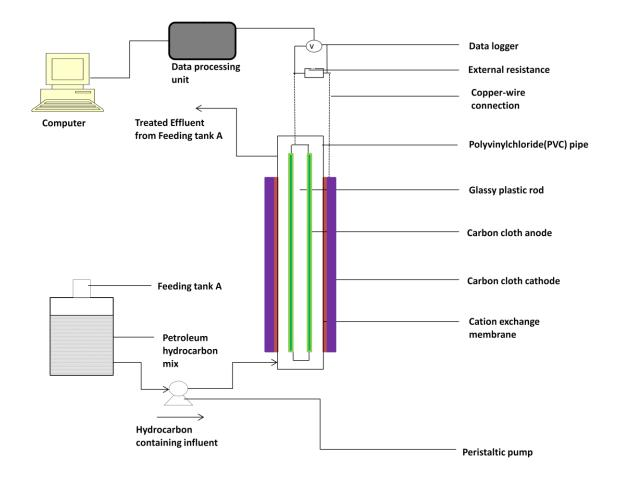
**Figure 2.3:** Schematic diagram of the tubular MFC reactor in an up-flow configuration used for the treatment of petroleum hydrocarbon containing synthetic wastewater for a possible *ex situ* application.
