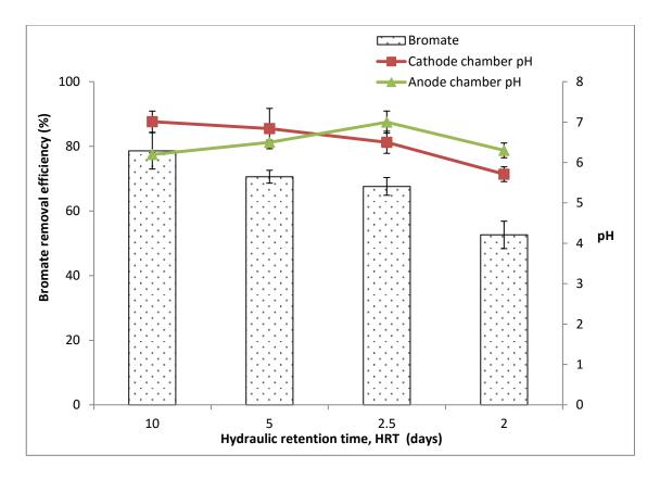
**Figure 5.4:** Bromate removal performances and changes in pH in the tubular MFC reactor over 110 days operation at ambient temperatures (10-25°C) using adapted microbial consortia. Error bars  $\pm$  SD are based on duplicate measurements.
