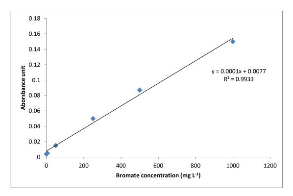
Figure 9.1: Calibration plot for bromate standard concentrations
