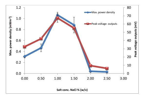
**Figure 4.2:** The effect of salinity on electrochemical performance of the MFC system at temp.  $30^{\circ}$ C using adapted anaerobic microbial consortia.. Values are means of duplicate experiments  $\pm$  SD.
