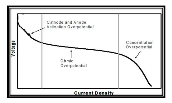
**Figure 1.16:** Regions of a polarisation curve used to assess the MFC performance depicting the energy losses (Image adapted from http://www.intechopen.com/source/html/16985/media/image17.png)
