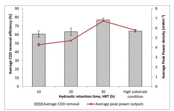
**Figure 5.8:** Average COD removal efficiencies and peak power densities generated as a function of time at different treatment conditions in a tubular MFC system over 100 days period of continuous operation using adapted microbial consortia. Values are means of duplicate experiments  $\pm$  SD.
