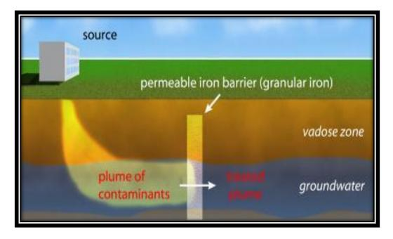
**Figure 1.12:** A typical conceptual design of a permeable reactive barrier (PRB) technology. (Source- https://commons.wikimedia.org/wiki/File:Iron\_Wall\_PRB.jpg).
