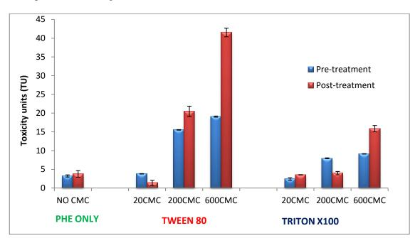
**Figure 4.9:** Toxicity response of two different surfactants at varying initial concentrations before and after treatment in a MFC using adapted microbial consortia as inoculum. The TU values are means of duplicate experiments  $\pm$  SD.
