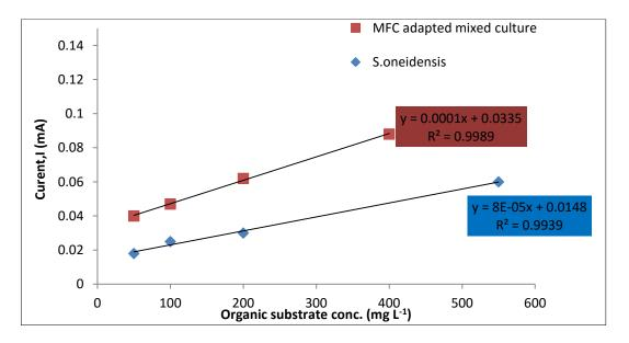
**Figure 3.13:** Relationship between organic substrate concentration and current generation from MFCs for different inocula (*S.oneidensis* and MFC-adapted mixed culture).
