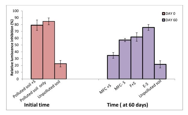
**Figure 6.9:** Toxicity levels in soil extractions of polluted soil with and without MFC treatment operated at 25-30°C over 60 days incubation period. The error bars represent 5% of deviation of the mean value for triplicate measurements. MFC-S and MFC+S are MFC only and MFC with surfactant (Tween 80, 250 mg  $L^{-1}$ ) amendment respectively. E-S and F+S mean controls without and with surfactant addition respectively.
