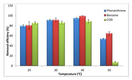
**Figure 4.4:** Effect of operating temperature on COD removal and degradation efficiencies during MFC operation using adapted anaerobic microbial consortia. Values are means of duplicate experiments  $\pm$  SD.
