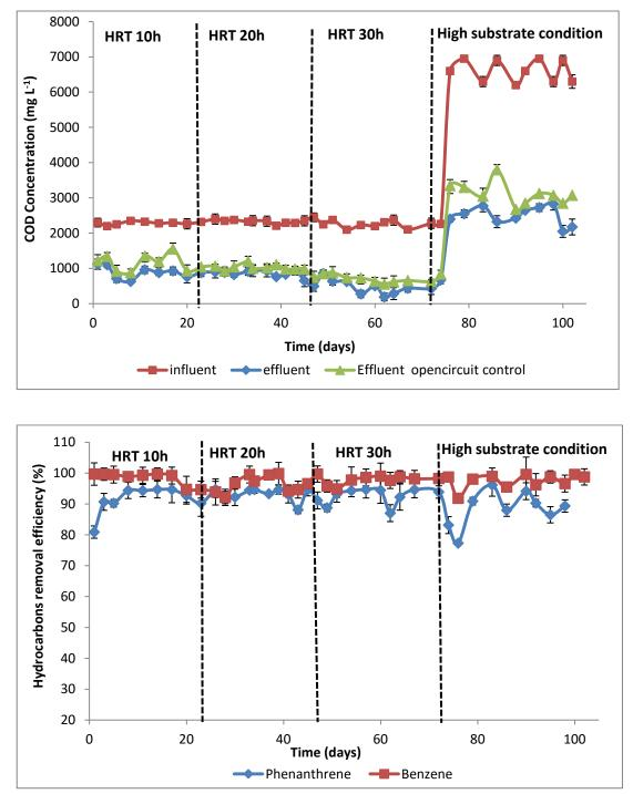
**Figure 5.7:** COD removal and hydrocarbons removal efficiencies at different HRTs and high substrate level condition at ambient temperatures (15-25°C) using adapted microbial consortia. Error bars  $\pm$  SD are based on duplicate measurements..
