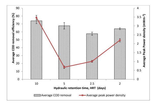
**Figure 5.3:** COD % removal and peak power density over the test period in MFCs at different HRTs in the tubular MFC at ambient temperatures (10-25°C) using adapted microbial consortia. Error bars  $\pm$  SD are based on duplicate measurements.
