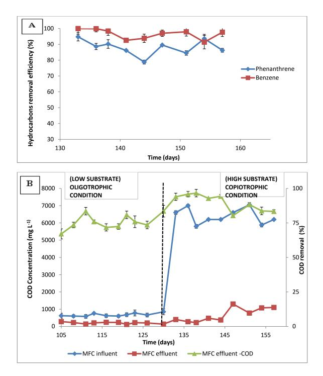
Figure 5.5: (A) Degradation performance of the tubular MFC at high substrate condition (B) COD removal at low and high substrate conditions operated in a continuous mode at HRT of 10 d. Error bars  $\pm$  SD are based on duplicate measurements.
