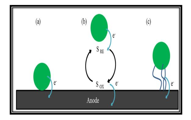
**Figure 1.15: Extracellular electron transfer mechanisms:** Microbially catalysed electron transfer from substrate reduction/oxidation onto electrode surface. This may occurs either through direct contact, mobile electron shuttles or nanowires respectively, as shown above (Chouler and Lorenzo, 2015).
