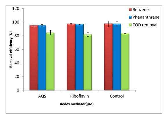
**Figure 4.5:** Effect of redox mediators on COD removal and degradation efficencies during MFC operation using adapted anaerobic microbial consortia. Values are means of duplicate experiments  $\pm$  SD.
