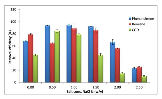
**Figure 4.3:** Effect of salt concentrations on COD removal and degradation efficencies during MFC operation (at  $30^{\circ}$ C) using adapted anaerobic microbial consortia. Values are means of duplicate experiments  $\pm$  SD.
