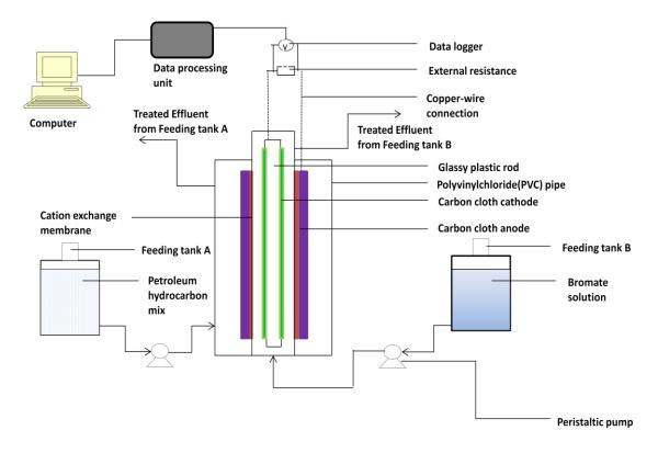
**Figure 2.2:** A schematic diagram of the tubular MFC reactor in an up-flow configuration for the treatment of hydrocarbon-containing synthetic wastewater for *in situ* applications.
