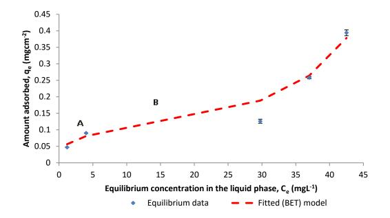
**Figure 3.1:** Adsorption isotherm of phenanthrene onto carbon felt [pH = 7; contact time = 180 mins; agitation speed: 0 rpm; adsorbent's surface area = 40 cm<sup>2</sup>, T = 30°C]. The error bars represent the SD of the mean.
