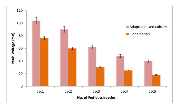
**Figure 3.11:** Comparison of peak voltages output of the two inoculum types (*S.oneidensis* MR1 and MFC-adapted mixed culture). Values are means of duplicate experiments  $\pm$  SD.
