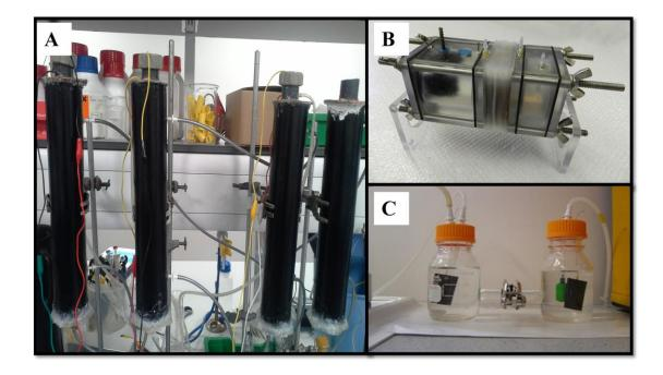
**Figure 1.17:** Types of dual chambered microbial fuel cells: (A) tubular up-flow type double chamber MFC systems with inner cathode for continuous flow operation (used in this study) (B) the rectangular type and (C) the conventional H-type two-chamber systems with large membrane surface areas (Logan et al., 2006).
