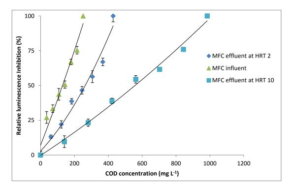
**Figure 5.6:** Bioluminescence based toxicity determinations of MFC effluent and influent at HRTs 10 and 2 days using bioluminescent marine bacteria, *V.fischeri*. Values are means of duplicate experiments  $\pm$  SD.
