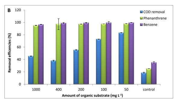
**Figure 3.12:** Removal efficiencies for degradation of phenanthrene and benzene using (A) *S.oneidensis* MR1 and (B) MFC-adapted mixed culture as inoculum respectively. Values are means of duplicate experiments  $\pm$  SD.
