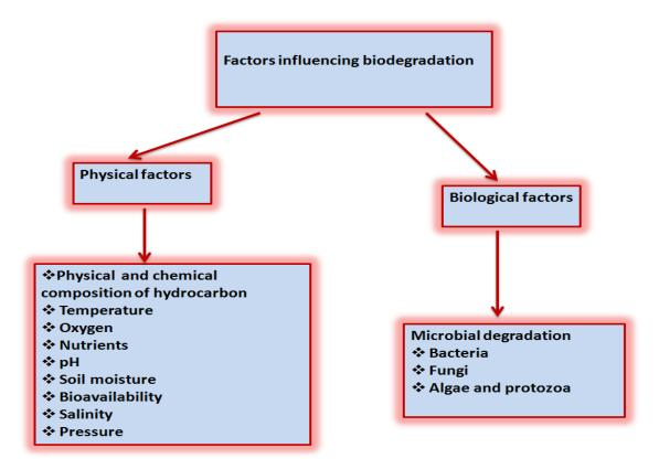
**Figure 1.7:** Environmental factors influencing the rate of biodegradation in the environment (Image adapted from Kriti and Chandra, 2014).
