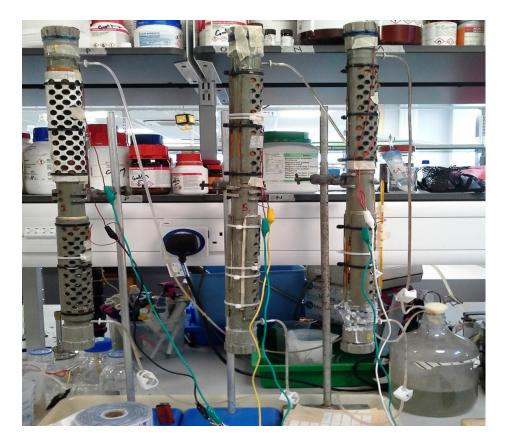
**Figure 9.4:** The MFC system (during start-up of the continuous run) used for the treatment of petroleum hydrocarbon containing synthetic wastewater.
