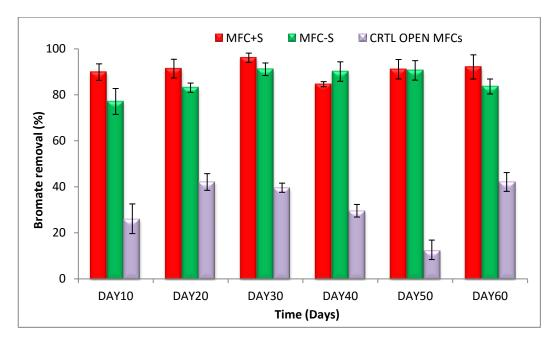
**Figure 6.5:** Bromate removal efficiency in the tubular MFC reactor during 60 days operation at incubation temperature between 25 and 30 °C. The error bars  $\pm$ SD were based on averages measured in triplicate.
