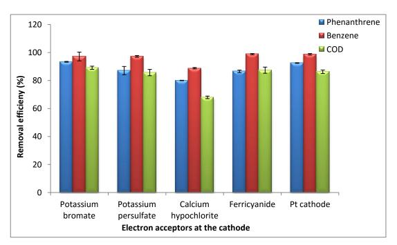
**Figure 4.6:** Effect of electron acceptors on COD removal and degradation efficiencies during MFC operation using adapted anaerobic microbial consortia. Values are means of duplicate experiments  $\pm$  SD.
