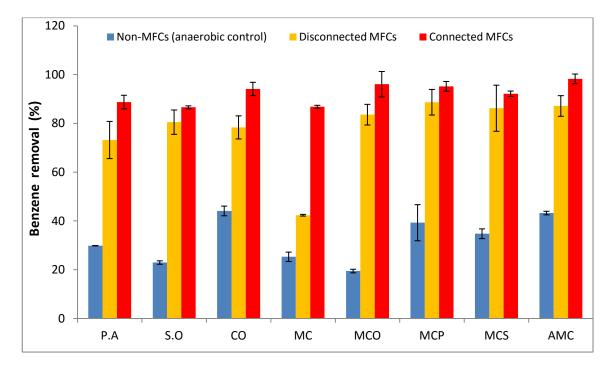
**Figure 3.8:** Degradation efficiencies for benzene removal by different inoculum types. *S. oneidensis* (S.O), *P. aeruginosa* (P.A), a co-culture of *S. oneidensis* and *P. aeruginosa* (CO), anaerobic digested sludge (MC), anaerobic digested sludge with the co-culture (MCO), anaerobic digested sludge with *S. oneidensis* (MCS), anaerobic digested sludge with *P. aeruginosa*, MCP and adapted mixed culture (AMC). The error bars represent the SD of the mean.
