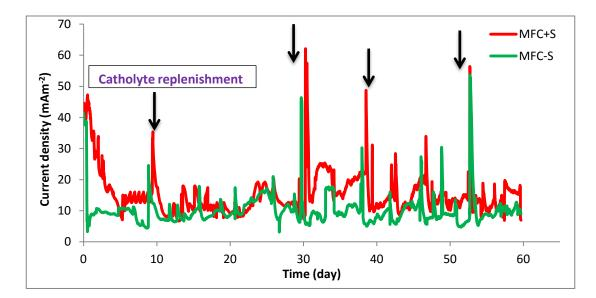
**Figure 6.6:** Current densities of MFC+S and MFC-S during the tubular MFC operations over 60 days incubation period ( $R_{ext} = 1000 \Omega$ ). Black arrows indicate the points for catholyte replenishment.
