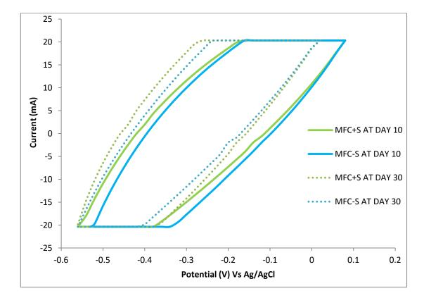
**Figure 6.7:** The CV curve for phenanthrene in MFC only (MFC-S) and MFC with surfactant (Tween 80, 250 mg  $L^{-1}$ ) amendment (MFC+S) at day 10 (solid line) and day 30 (dashed line) at sweep rate of 10 mVs<sup>-1</sup>.
