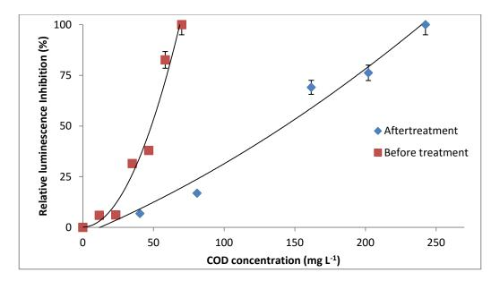
**Figure 3.10:** *Vibrio fischeri* bioluminescence based toxicity determinations of pretreated and treated samples from MFC seeded with MFC-adapted mixed culture (at 200 mg L<sup>-1</sup> benzene concentration). Values are means of duplicate experiments  $\pm$  SD.
