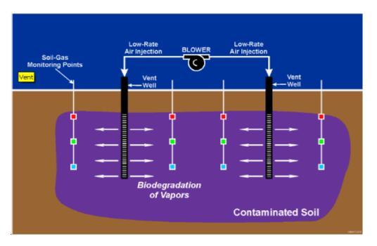
**Figure 1.11:** A typical representative design for bioventing and biosparging systems (Garima and Singh, 2014).
