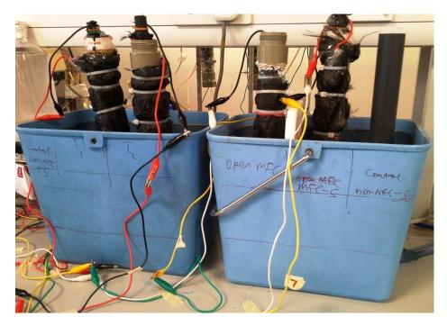
Figure 9.3: (A) The soil MFC system during start-up for treating a model PAH-contaminated soil
