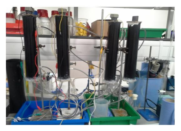
**Figure 9.2:** The experimental set-up during the start-up stage of the continuous run of the tubular MFC system for the treatment of synthetic wastewater containing petroleum hydrocarbons.
