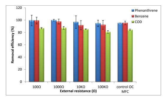
**Figure 4.10:** Degradation and COD reduction performance of MFC systems at various external resistances compared to open circuit control during 10 days of operation using adapted mixed culture at incubation temperature of  $30\pm3^{\circ}$ C.. Values are means of duplicate experiments  $\pm$  SD.
