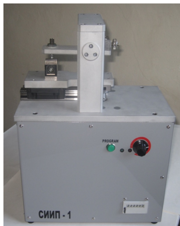
Fig. 2. General view of a SIIP stand for testing wear resistance
