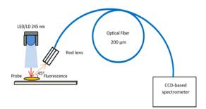
Fig. 1. Mobile experimental installation used by fluorescence spectroscopy
