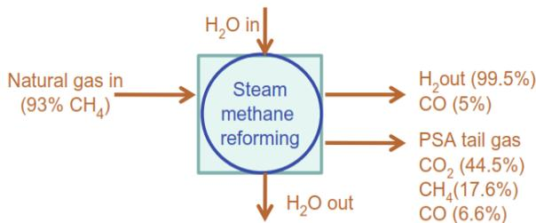
**Figure 1.** Block diagram of the steam methane reforming process [14]. In the first stage of the process, a catalytic endothermic reaction (Eq. 1) takes place between methane (natural gas) and steam at a high temperature (the steam methane reforming process). As a result of this reaction, synthesis gas is produced, which contains 85% of carbon monoxide, hydrogen, and small amounts of residual methane and carbon dioxide and water [15].
