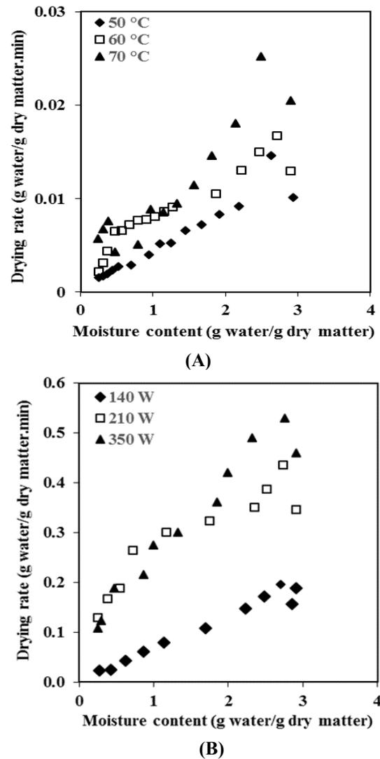
**Figure 2.** Drying rates *versus* moisture content of sour cherry samples at different temperatures (A) and power levels (B)
