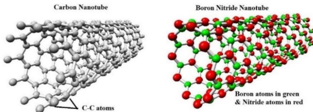
**Figure 1.** Structure of CNT and BNNT
