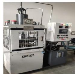
**Figure 5.** Compression moulding machine
