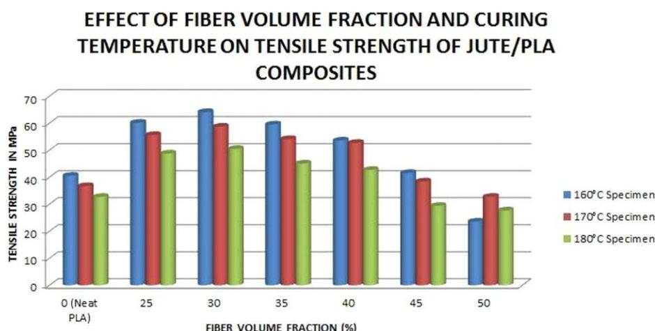
**Figure 6.** Effect of fiber volume fraction and curing temperature on tensile strength of Jute/PLA composites (open access) [78]
