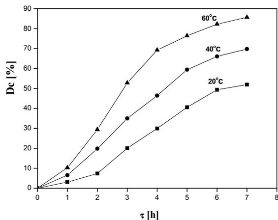
Fig. 3. Relationships between degree of conversion and time on stream at different temperatures:  $T = 20, 40$  and  $60^\circ\text{C}$ ; electrolyte:  $15 \text{ g S}^{2-}\cdot\text{l}^{-1} + 0.25 \text{ N NaOH} + \text{O}_2$  (Air); non-modified GDE;  $\text{SGDE} = 200 \text{ cm}^2$ ; flow rate  $v_r = 24.15 \text{ cm}^3\cdot\text{min}^{-1}$ .
