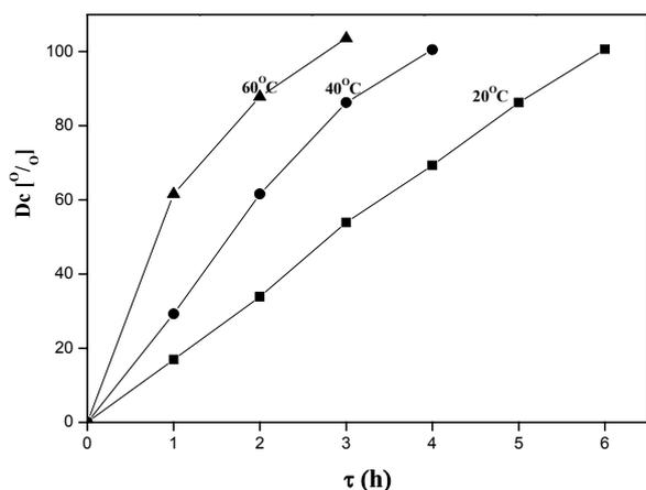
Fig. 6. Relationships between degree of conversion and time on stream at different temperatures for Ni(OH)<sub>2</sub> catalyst on GDE: SGDE = 200 cm<sup>2</sup>; T = 20, 40 and 60°C; electrolyte: 15 g S<sup>2-</sup>·l<sup>-1</sup> + 0.25 N NaOH + O<sub>2</sub> (Air); flow rate  $v_f = 24.15 \text{ cm}^3 \cdot \text{min}^{-1}$ .
