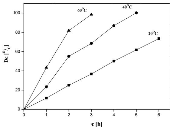
Fig. 5. Relationships between degree of conversion and time on stream at different temperatures for CoPc(SO<sub>3</sub>H)] catalyst on GDE: SGDE = 200 cm<sup>2</sup>; T = 20, 40 and 60°C; electrolyte: 15 g S<sup>2-</sup>·l<sup>-1</sup> + 0.25 N NaOH + O<sub>2</sub> (Air); flow rate  $v_f = 24.15 \text{ cm}^3 \cdot \text{min}^{-1}$ .
