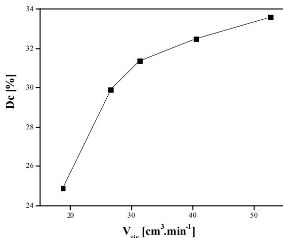
Fig. 2. Relationship between rate of sulphide oxidation by oxygen and flow rate of solution;  $T = 20^\circ\text{C}$ ; electrolyte:  $15 \text{ g S}^{2-}\cdot\text{l}^{-1} + 0.25 \text{ N NaOH}$ ; non-modified GDE  $\text{SGDE} = 200 \text{ cm}^2$ .
