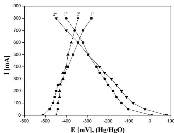
Fig. 7. Partial polarization curves: T = 20°C; flow rate  $v_f = 24.15 \text{ cm}^3 \cdot \text{min}^{-1}$ ; SGDE = 200 cm<sup>2</sup>; cathodic curves: (15 g S<sup>2-</sup>·l<sup>-1</sup> + 0.25 N NaOH + Ar), (●) - [CoPc(SO<sub>3</sub>H)<sub>2</sub>] and (▼) - Ni(OH)<sub>2</sub>; anodic curves (0.25 N NaOH + O<sub>2</sub> (Air)), (■) - [CoPc(SO<sub>3</sub>H)<sub>2</sub>] and (▲) - Ni(OH)<sub>2</sub>;
