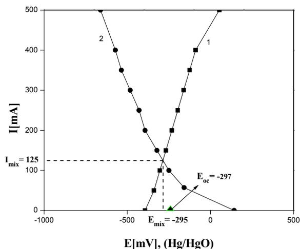
Fig. 4. Partial polarization curves:  $T = 20^\circ\text{C}$ ; non-modified GDE;  $v_r = 24.15 \text{ cm}^3\cdot\text{min}^{-1}$ ;  $\text{SGDE} = 200 \text{ cm}^2$ ; cathodic curve (■) -  $15 \text{ g S}^{2-}\cdot\text{l}^{-1} + 0.25 \text{ N NaOH} + \text{Ar}$ ; anodic curve (●) -  $0.25 \text{ N NaOH} + \text{O}_2$  (Air);  $E_{oc}$  (▲) -  $15 \text{ g S}^{2-}\cdot\text{l}^{-1} + 0.25 \text{ N NaOH} + \text{O}_2$  (Air).
