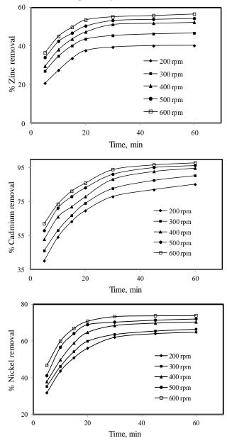
**Fig 6**. The effect of stirring speed on removal efficiency (pH 6.0, 1 g/500 ml resin dosage, 293 K solution temperature and 250 mg  $L^{-1}$  initial metal concentration).
