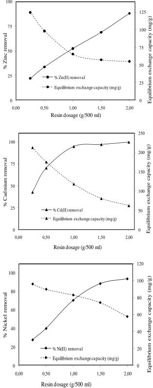
**Fig. 5a.** The effect of resin dosage on removal efficiency and exchange capacity (pH 6.0, 293 K solution temperature, 400 rpm stirring speed and 250 mg  $L^{-1}$  initial metal concentrations).
