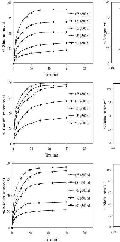
**Fig. 5**. The effect of resin dosage on removal efficiency (pH 6.0, 293 K solution temperature, 400 rpm stirring speed and 250 mg  $L^{-1}$  initial metal concentrations).
