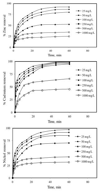
**Fig. 3.** The effect of initial metal concentration on removal efficiency (pH 6.0, 293 K solution temperature, 400 rpm stirring speed, 1 g/500 ml resin dosage).
