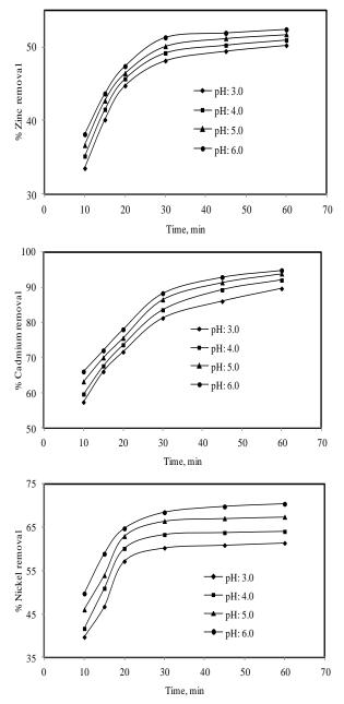
**Fig. 2.** The effect of initial pH on removal efficiency for the here metal ions (250 mg  $L^{-1}$  initial metal concentration, 293 K solution temperature, 400 rpm stirring speed, 1 g/500 ml resin dosage).
