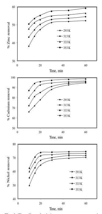
Fig. 4. The effect of solution temperature on removal efficiency (pH 6.0, 1 g/500 ml resin dosage, 400 rpm stirring speed and 250 mg  $L^{-1}$  initial metal concentrations).
