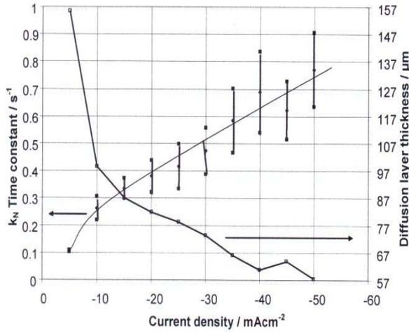
**Fig. 18.** Current density dependence of the diffusion time constant (2<sup>nd</sup> parameter of  $Z_N$ ) and calculated diffusion layer thickness during oxygen reduction reaction on Ag-GDE in 10 N NaOH, 80°C.
