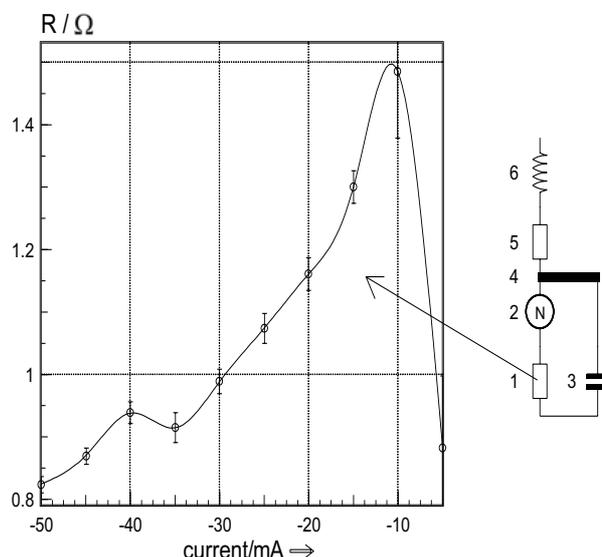
**Fig. 13.** Current density dependence of the charge transfer resistance (element number 1) during oxygen reduction reaction on Ag-GDE in 10 N NaOH, 80°C.
