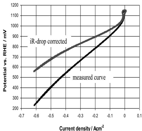
**Fig. 9.** Uncorrected and  $iR_{el}$  corrected data of the CV recorded with 1 mV/s at 80°C during ORR in 10 N NaOH in the potential range from OCP to 230 mV vs. RHE (-700 mV vs. Hg/HgO)
