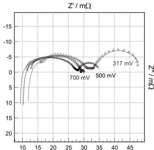
**Fig. 3.** Nyquist diagram of selected EIS measured on PEFC at low cell voltages, 80°C, at 2 bar absolute, at different cell voltages (currents): (o) 700 mV (5.4 A), (□) 500 mV (12.1 A) and (Δ) 317 mV (17.5 A).
