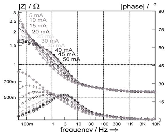
**Fig. 11.** Bode representation of impedance spectra measured at different current densities during oxygen reduction reaction on Ag-GDE in 10 N NaOH, 80°C.
