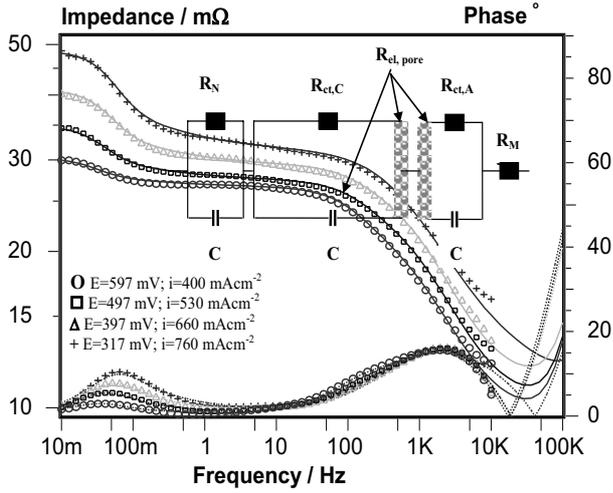
**Fig. 4.** Bode diagram of EIS measured in the low cell voltage range, at 80°C, at 2 bar absolute, at different cell voltages (currents): (o) 597 V, (□) 497 mV, (Δ) 397 mV and (+) 317 mV with the schematic representation of the used EC for fitting as insert.
