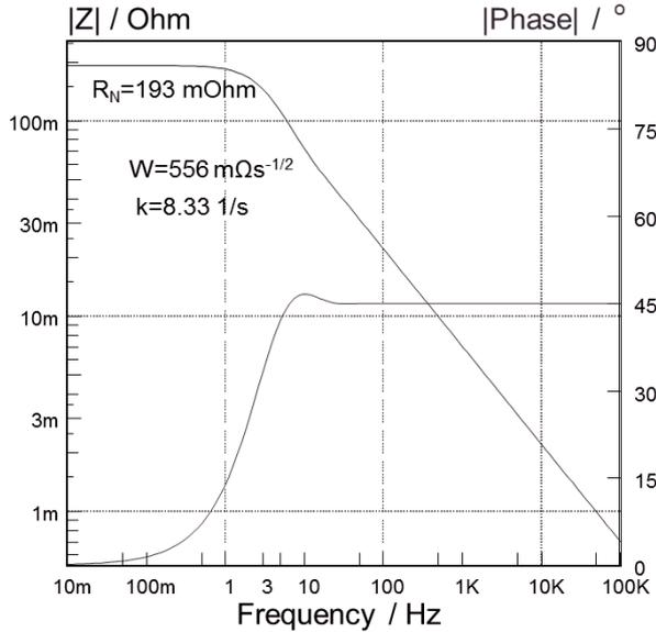
**Fig. 19.** Bode diagram of simulated impedance spectra of the Nernst impedance  $Z_N$  with  $W=556 \text{ m}\Omega\text{s}^{-1/2}$  and  $k_N=8.33 \text{ s}^{-1}$ .
