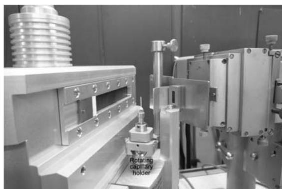
Fig. 2. Rotating capillary setup
