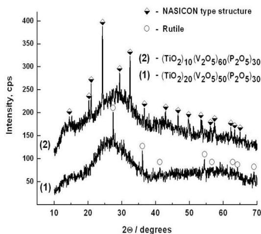
**Fig. 1.** X-ray diffraction patterns of (TiO<sub>2</sub>)<sub>20</sub>(V<sub>2</sub>O<sub>5</sub>)<sub>50</sub>(P<sub>2</sub>O<sub>5</sub>)<sub>30</sub> and (TiO<sub>2</sub>)<sub>10</sub>(V<sub>2</sub>O<sub>5</sub>)<sub>60</sub>(P<sub>2</sub>O<sub>5</sub>)<sub>30</sub> samples.
