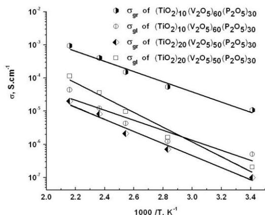
**Fig. 3** Arrhenius plots of the conductivities of (TiO<sub>2</sub>)<sub>20</sub>(V<sub>2</sub>O<sub>5</sub>)<sub>50</sub>(P<sub>2</sub>O<sub>5</sub>)<sub>30</sub> and (TiO<sub>2</sub>)<sub>10</sub>(V<sub>2</sub>O<sub>5</sub>)<sub>60</sub>(P<sub>2</sub>O<sub>5</sub>)<sub>30</sub> glass-crystalline samples.
