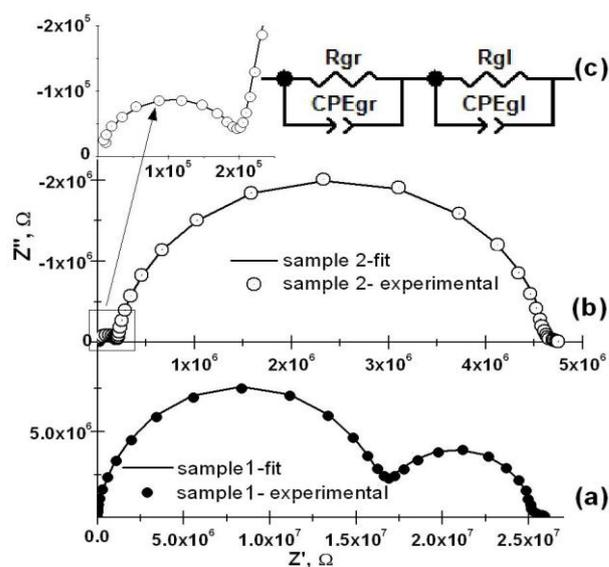
**Fig. 2.** Nyquist plots of (a) (TiO<sub>2</sub>)<sub>20</sub>(V<sub>2</sub>O<sub>5</sub>)<sub>50</sub>(P<sub>2</sub>O<sub>5</sub>)<sub>30</sub>; (b) (TiO<sub>2</sub>)<sub>10</sub>(V<sub>2</sub>O<sub>5</sub>)<sub>60</sub>(P<sub>2</sub>O<sub>5</sub>)<sub>30</sub> samples and (c) equivalent circuit.
