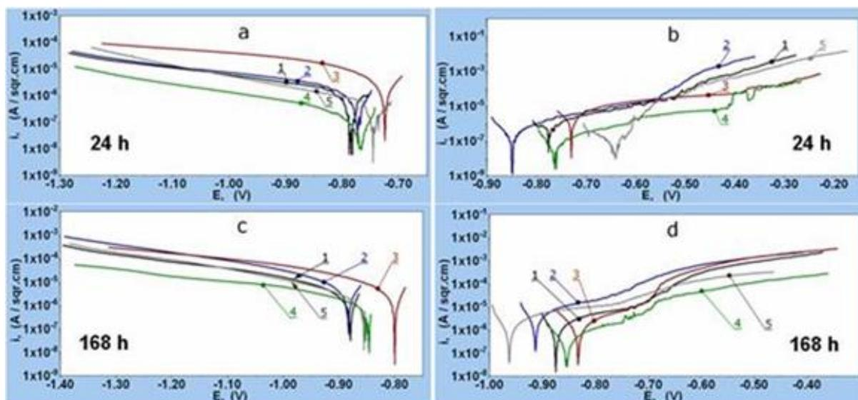
**Fig. 4.** LSV-curves of the samples acquired after 24 (a) and 168 (b) hours of exposition to 3.5% NaCl model corrosive medium. 1 – sample P1; 2 – sample P2, 3 – sample P3, 4 – sample P4, 5 – sample P5,
