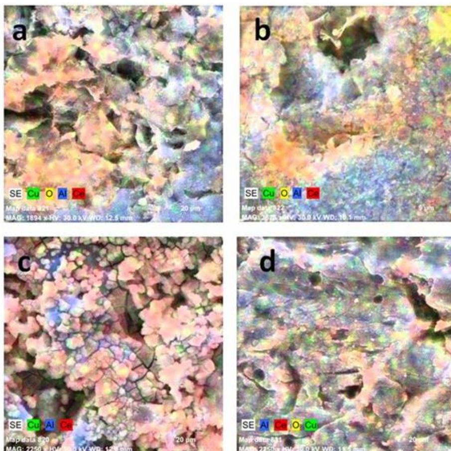
**Fig. 6.** EDS topological images of the investigated samples: a – specimen P1; b – specimen P2; c – specimen P3; d – specimen P4
