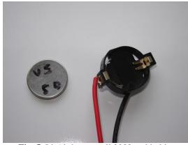
Fig. 5. Li-Air button cell 2032 and holder
