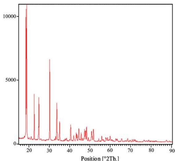
Fig. 2. XRD pattern of the ZnO nanoparticles.
