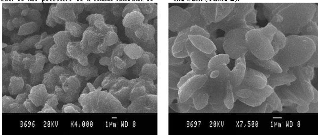
Fig. 3. Scanning electron microscopy (SEM) image of the synthesized ZnO nanoparticles.
