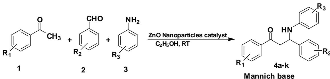
Scheme 1. Synthesis of  $\beta$ -amino carbonyl compounds from amines, acetophenone and aldehydes catalyzed by ZnO nanoparticles catalyst
