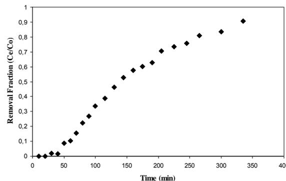
**Fig. 6.** Boron removal in the fixed bed reactor
