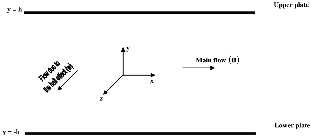
Fig. 1. Schematic diagram of the system.
