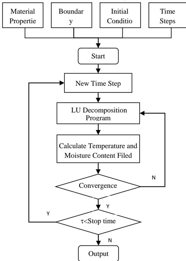
Fig. 2. Flow chart of the numerical calculation.
