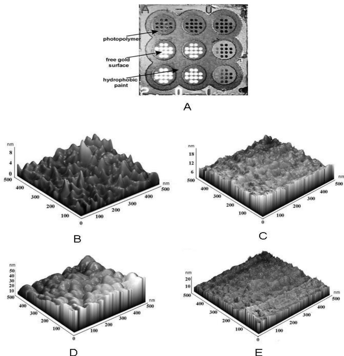
**Fig. 1.** Picture of chip (A) and AFM pictures of bare gold (B), thiol (cysteamine 20 mM) (C), podoplanin antibody (1.5 µg/ml) (D), thiol after regeneration (E). Initial antibody concentration: 1.5 µg/ml. Initial podoplanin concentration: 1 ng/ml.
