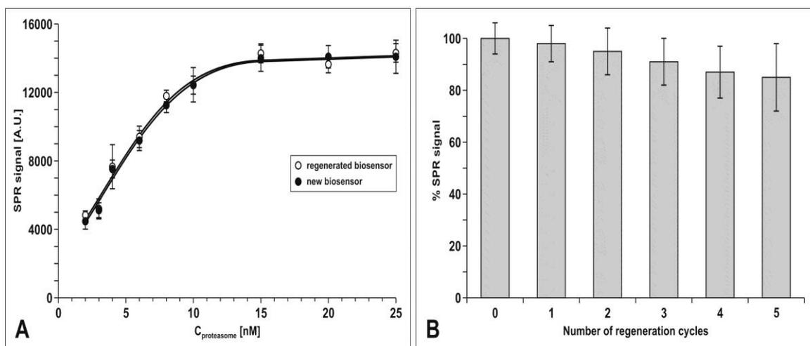
**Fig. 2.** (A) Dependence of SPR signal (Arbitrary Units) on proteasome 20S concentration for the PSI inhibitor (80 nM) (B) Effect of repeated chip regeneration on the proteasome 20S SPR signal on the PSI inhibitor. Concentration of proteasome 20S: 6 nM. pH value of proteasome solution: 7.4.
