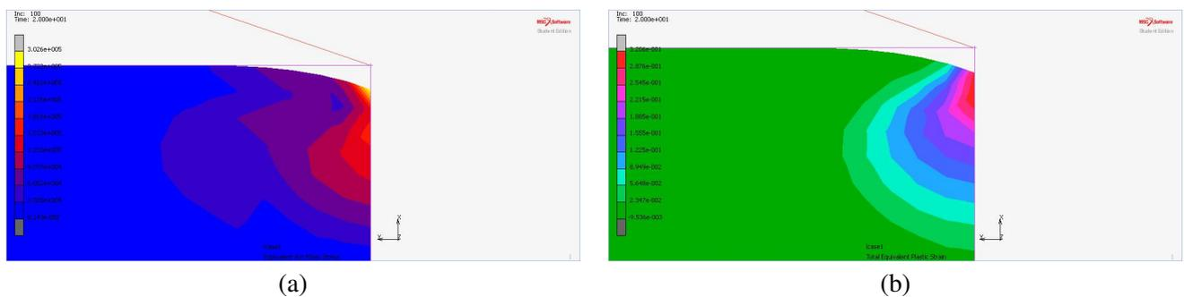
Fig. 11. Distribution of equivalent Von Mises stress (a) and the equivalent plastic strain (b) in material 2.
