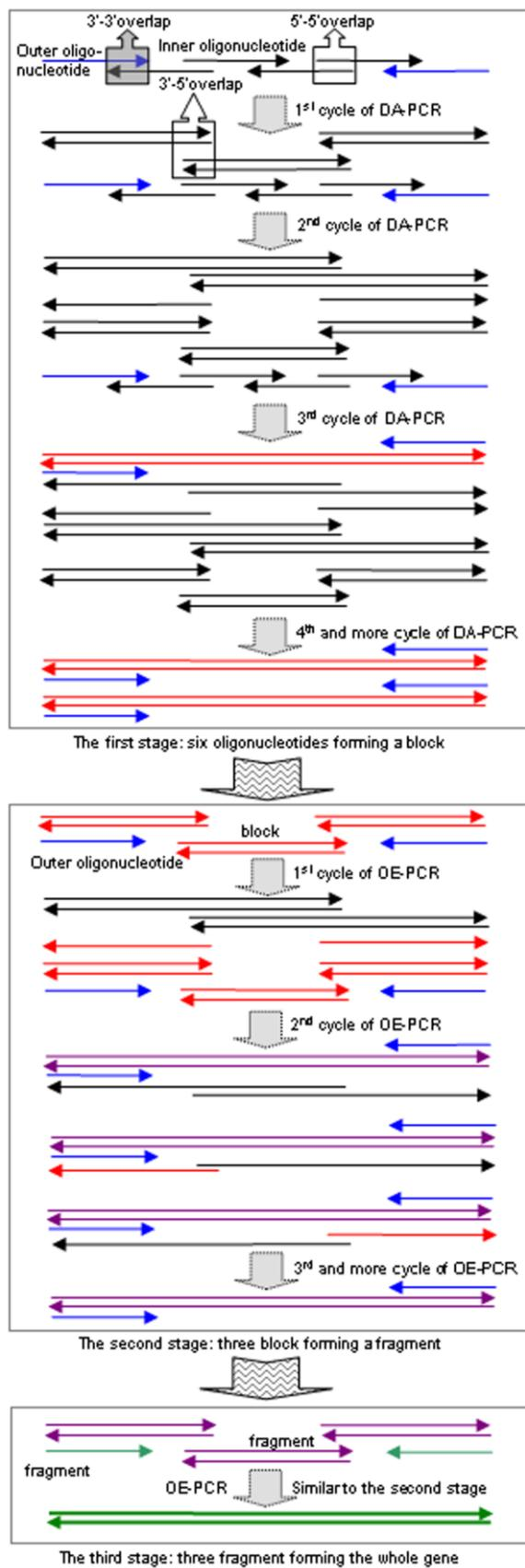
**Fig. 1.** Schematic diagram of the three-stage assembling method.
