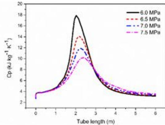
Fig. 6. Curves of specific heat of the fluid near the wall.
