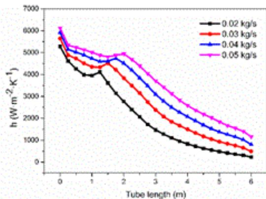
Fig. 5. Curves of surface heat transfer coefficient.
