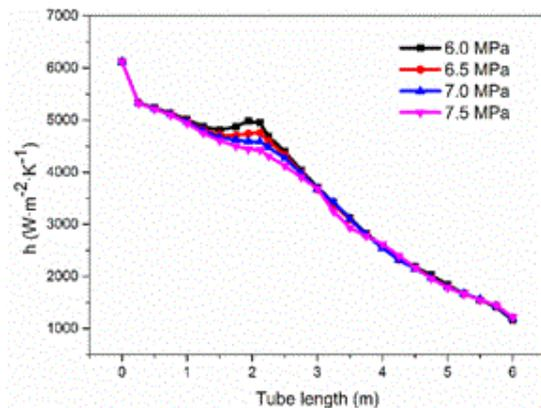
Fig. 7. Curves of surface heat transfer coefficient.
