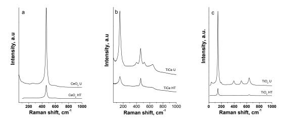
**Fig. 2.** Raman spectra of  $CeO_2$  (a), TiCe (b) and TiO<sub>2</sub> (c) materials.
