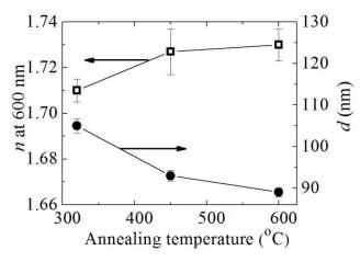
**Fig. 4.** Refractive index (*n*) at wavelength of 600 nm and thickness (*d*) of Nb<sub>2</sub>O<sub>5</sub> films prepared with PEO-*b*-PDMAA template as a function of postdeposition annealing temperature
