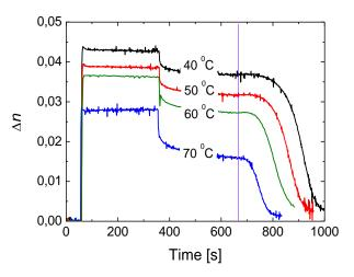
**Fig. 2.** Birefringence values during recording and thermal erasure. Recording temperatures are: 40°C, 50°C, 60°C, 70°C. The vertical line at 660 seconds indicates the start of temperature increase.
