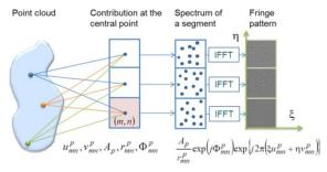
**Fig. 3.** Schematic of the accelerated computation of fringe patterns for elemental holograms.
