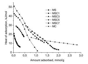
Fig. 4. Heats of adsorption for CO<sub>2</sub>.
