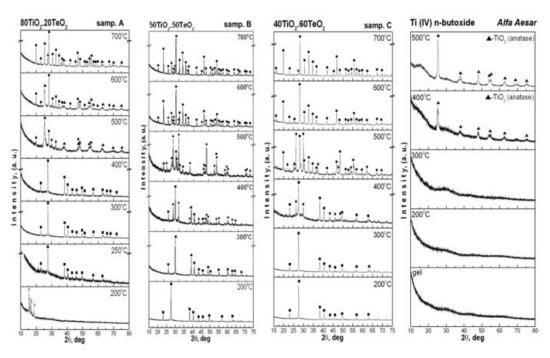
(**I**) Te, ( $\blacklozenge$ )  $\alpha$ -TeO<sub>2</sub>, (**A**) TiO<sub>2</sub>-anatase, ( $\ast$ ) TiO<sub>2</sub>-rutile, ( $\bullet$ ) TiTe<sub>3</sub>O<sub>8</sub>, ( $\odot$ ) H<sub>3</sub>BO<sub>3</sub>, ( $\diamondsuit$ ) ZnTiO<sub>3</sub> (rhomb).
