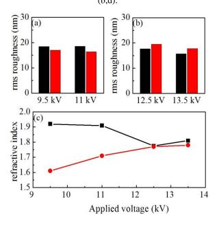
**Fig. 4.** Surface roughness (rms) in [nm] of ZnO films deposited at emitter-to-collector distance of 4 cm (a) and 7 cm (b) and refractive index at wavelength of 600 nm as a function of applied voltage (c) for as-deposited (black color) and annealed films (red color).
