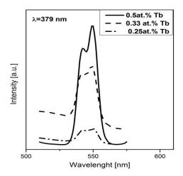
**Fig. 4.** The emission spectra of samples with different terbium ion concentration.
