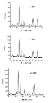
Fig. 1. XRD spectra of  $BaFe_{12}O_{19}$  powders: (a) - YLT1A, (b) - YLT1B, (c) - YLT1C.
