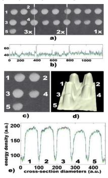
Fig. 7. (a) The plot of the parts of sheets under investigation A1x-A3x with registered spots; (b) the line of blackness for the different sheets; (c) the spots on the sheet A3x in increased scale and their (d) 2D and (e) 3D computer processing obtained images.
