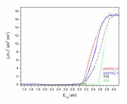
Fig. 3. Band gap energy  $E_{bg}$  of TiO<sub>2</sub> P25 Degussa, and mechanochemically synthesized ZnS, ZnS/TiO<sub>2</sub>-1 and ZnS/TiO<sub>2</sub>-2 samples.
