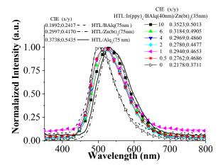
Fig. 4. Normalized electroluminescence spectra of devices HTL/Balq(75nm), HTL/Zn(bt)2(75nm), HTL/Alq3(75nm), and HTL:Ir(ppy)3(x wt.%)
