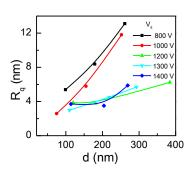
**Fig. 7.** Standard deviation  $R_{a}$  of surface roughness as a function of the thickness of ITO films, deposited at indicated V<sub>s</sub>.
