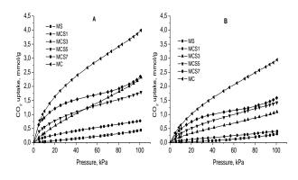
**Fig. 3.** CO<sub>2</sub> adsorption isotherms at: A - 0 °C and B -30 °C for various mesoporous silica-carbon composites.
