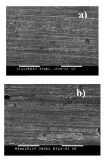
**Fig. 2.** SEM images of as-received archwire 0.017x0.025 inches<sup>2</sup> (a) and 0.019x0.025 inches<sup>2</sup> (b)
