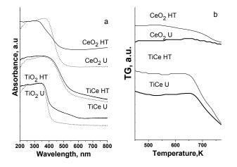
**Fig 3.** UV-Vis spectra (a), TPR–TG profiles (b) of TiCe materials.
