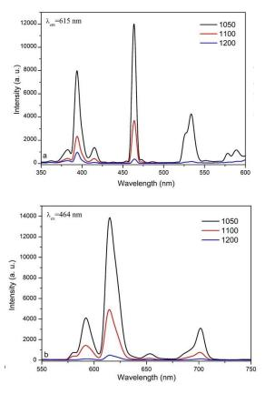
**Fig. 6.** PL (a) excitation and (b) emission spectra of  $55B_2O_3 \cdot 35Bi_2O_3 \cdot 10La_2O_3 : Eu^{3+}$  glass and glass-crystal samples obtained by melt quenching technique at different temperatures.
