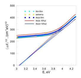
**Fig. 1.** Tauc plot for 0.01 M oxalic acid concentration. The results shown by circles are calculated from expressions for thin film, the boxes are from formulae
