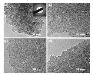
Fig. 1. TEM pictures of Nb<sub>2</sub>O<sub>5</sub> thin films prepared using 5 wt % PDMAA-b-PEO (a), PDMAA-b-PEO-b-PDMAA (b), PDMAA (c) and PEO (d) as organic template (ratio polymer to NbCl<sub>5</sub> equals to 0.23) and annealed at 320 °C for 30 min. The inset shows Selected Area Electron Diffraction pattern.
