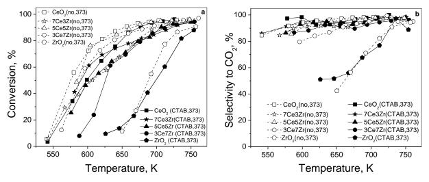
Fig. 5. Temperature dependency of ethyl acetate total oxidation for the studied samples.
