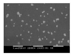
Fig. 4. SEM image of vacuum deposited ZnPc film. Thickness: 75±2 nm.
