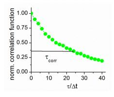
Fig. 5. Normalized temporal correlation function (the abscissa gives the ratio between the time lag and the acquisition interval  $\Delta t = 250$  ms).
