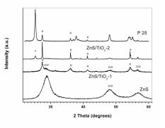
**Fig. 1.** XRD patterns of initial TiO<sub>2</sub> P25 Degussa and mechanochemically synthesized samples ZnS, ZnS/TiO<sub>2</sub>-1 and ZnS/TiO<sub>2</sub>-2.
