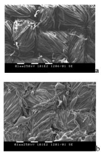
**Fig.3.** SEM micrographs of the surface morphology of non-impregnated (a) and PET impregnated textile (b).
