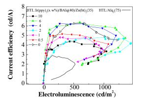
**Fig. 6.** Current efficiency as a function of electroluminescence of devices HTL:Ir(ppy)<sub>3</sub> (x wt.%)/BAlq(40nm)/Zn(bt)<sub>2</sub> (35nm) and HTL/Aq<sub>3</sub>(75nm).
