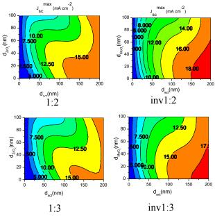
**Fig. 7.** Calculated short-circuit current density  $J_{sc}^{max}$  contours under 100 mW cm<sup>-2</sup> AM 1.5G spectral illumination as a function of active layers and optical spacer thicknesses for: a) standard device with ZrO<sub>2</sub> optical spacer and b) inverted device with MoO<sub>3</sub> optical spacer.
