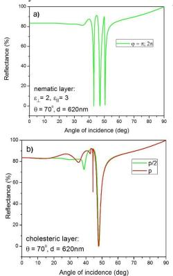
**Fig. 2**. Reflection spectra of p- polarized light as a function of incident angle for structures with a) nematic and b) cholesteric layer. All other parameters of the structures are identical.
