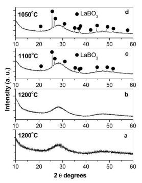
**Fig. 1.** XRD patterns of  $55B_2O_3 \cdot 35Bi_2O_3 \cdot 10La_2O_3$  (a) and  $55B_2O_3 \cdot 35Bi_2O_3 \cdot 10La_2O_3$  : Eu<sup>3+</sup> (b-d) glass and glass-crystalline samples obtained by melt quenching at different temperatures.
