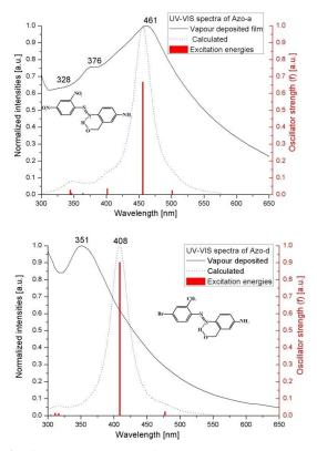
**Fig. 1.** UV-VIS spectra of Azo-a and Azo-d as vapour deposited nanosized films and theoretically calculated by TD-DFT/ B3LYP 6-31+G(d,p) level of theory in vacuo.
