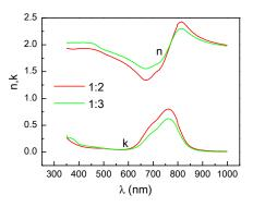
**Fig. 4.** Refractive index (n) and extinction coefficient (k) spectra of blended Sq1/PC<sub>61</sub>BM films.
