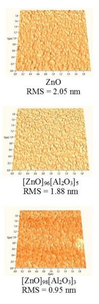
Fig. 4. AFM of ZnO and Al-doped ZnO (AZO).
