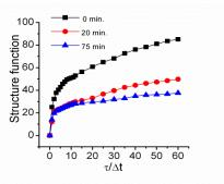
**Fig. 5** Structure function of intensity fluctuations in the center of the drop pf PAZO water solution at three time offsets.).
