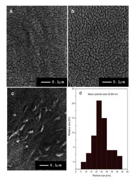
Fig. 4. SEM micrographs of the glass and different part of the glass-ceramic treated at 560°C during 4 hours: (a) – glass, (b) – center of the glass-ceramic, (c) – edge of the glass-ceramic and (d) - particle distribution and average particle size of the same glass-ceramic.
