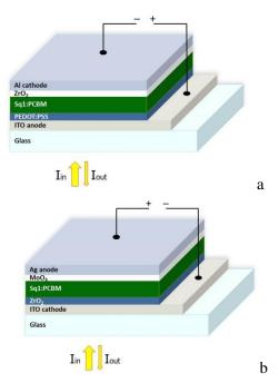
**Fig. 1.** Scheme of BHJ organic solar cells with: a) standard structure; b) inverted structure.
