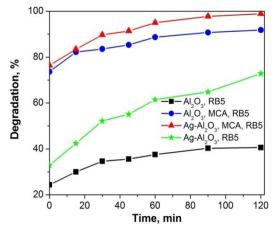
**Fig. 4.** Degree of degradation of RB5 dye as a function of the time of UV illumination.
