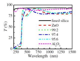
**Fig. 3.** Transmittance spectra of Al<sub>2</sub>O<sub>3</sub>, ZnO and samples with compositions ZnO: Al<sub>2</sub>O<sub>3</sub> (cycles ratio shown)
