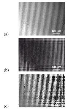
Fig. 3. Images of diffraction grating with spatial frequency of 100 lines/mm recorded in Bayfol HX200 photopolymer: a) a digital hologram; b) reconstructed intensity at 2  $\mu$ m depth inside the photopolymer layer; c) reconstructed phase at 2  $\mu$ m depth inside the photopolymer layer.
