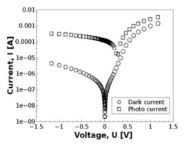
**Fig. 7.** *I-V* characteristics of ITO|PEDOT:PSS| ZnPc:C<sub>60</sub>|Al samples measured in dark and under light exposure with light according to standard AM 1.5.
