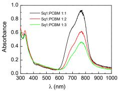
**Fig. 2.** Absorption spectra of 100 nm thick Sq1/PC<sub>61</sub>MB films with different D/A weight ratio.
