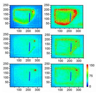
**Fig. 4.** 2D distribution of the temporal structure function at time offsets 0 minutes (top), 20 minutes (middle) and 75 minutes (bottom); left -  $\tau = 10\Delta t$ , right -  $\tau = 50\Delta t$ .
