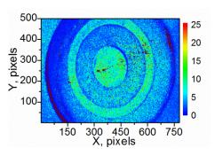
Fig. 7. Contour map of the normalized temporal correlation function at a time lag  $\tau = 5\Delta t$ ; the time scale is given in seconds.
