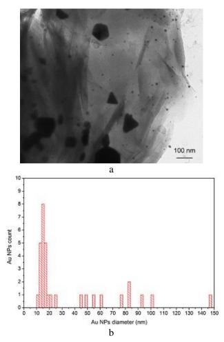
Fig. 2. a) TEM image with 50 000 times magnification of the sample after UV treatment; b) Histogram showing size distribution of 32 gold nanoparticles observed in Fig. 2a.
