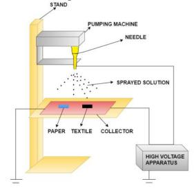
Fig. 1. Design of electrospinning/electrospraying apparatus.
