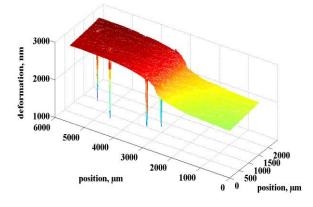
**Fig. 5.** Two dimensional distribution of the deformation filed due to temperature change from 32 °C to 50 °C.
