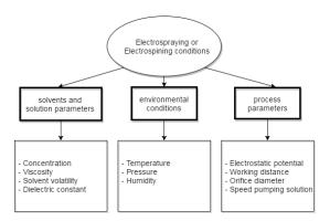
Fig. 2. The electrospraying or electrospinning conditions.
