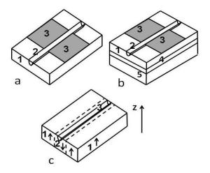
Fig. 1. A principle scheme of a phase shifter (a); PELN on insulator phase modulator (b): 1 – substrate, 2 – PE stripe waveguide, 3- electrodes, 4 – SiO<sub>2</sub> layer; schematic representation of a dipole inverted PE element for electric field sensor (c): 1, 2 – DI regions, 3 – PE stripe
