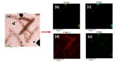
Fig. 6. (a,b,c,d,e). (a) Integral XEDS-STEM composition map from carbon rich area of sample C heat treated at 400°C; (b) composition map of Te; (c) composition map of Ti; (d) composition map of C; (e) composition map of O.
