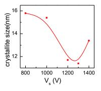
Fig. 4. Crystalite size of 180 nm thick ITO films as a function of sputtering voltage.
