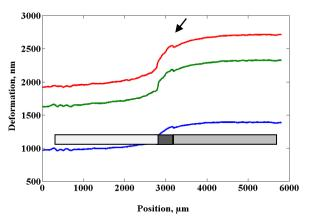
**Fig. 6.** Cross-sections of deformation at different moments of thermal load at 40 <sup>o</sup>C – blue line, 48 <sup>o</sup>C – green line and 51 <sup>o</sup>C – red line.
