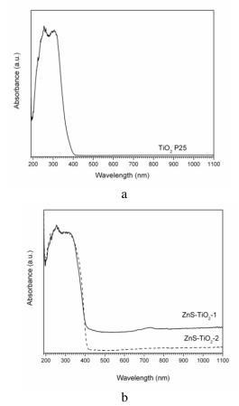
**Fig. 2.** UV-vis absorbance spectrum of: a) TiO<sub>2</sub> P25 Degussa; b) mechanochemically synthesized ZnS/TiO<sub>2</sub> composites.
