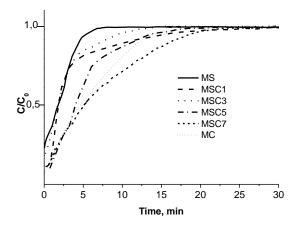
Fig. 5.  $CO_2$  capture curves (0.3 vol%  $CO_2$ , 10 ml/min,  $45^{\circ}C$ ).
