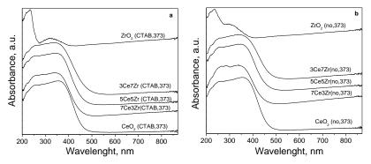
Fig. 3. UV-Vis spectra for the samples prepared with CTAB template (a) and without (b)
