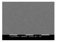
Fig. 3. SEM image of vacuum deposited C60 film. Thickness: 45±3 nm.
