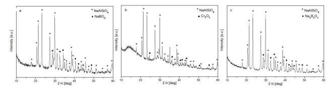
**Fig. 2.** XRD patterns of the glass-ceramic obtained from glass composition numbered from 5 to 7. (a) – composition 5 treated at 550°C 16h; (b) - composition 6 treated at 550°C 12h; (c) composition 7 treated at 580°C 8h.
