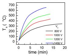
**Fig. 2.** Variation of the substrate temperature T<sub>s</sub> with the deposition time at indicated sputtering voltages.
