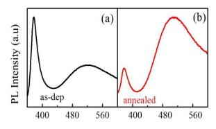
**Fig. 5**. Room temperature photoluminescence spectra of as-deposited (a) and annealed (b) ZnO films taken at excitation wavelength of 335 nm.
