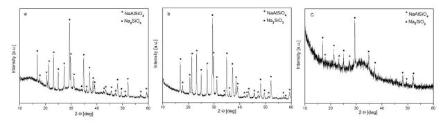
**Fig. 1.** XRD patterns of the glass-ceramics obtained from the glass compositions numbered 1, 2 and 4 treated at 700°C 24h (a), 600°C 24h (b) and 600°C 16h (c) respectively.
