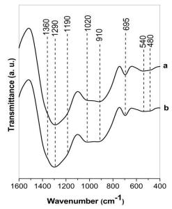
**Fig. 2.** IR spectra of  $55B_2O_3 \cdot 35Bi_2O_3 \cdot 10La_2O_3$  (a) and  $55B_2O_3 \cdot 35Bi_2O_3 \cdot 10La_2O_3$  : Eu<sup>3+</sup> (b) glass samples obtained by melt quenching technique.
