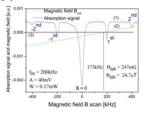
Fig. 3. Dark resonances in K vapor absorption measured as a function of magnetic field B, scanned around B = 0. The measured stray magnetic field in laboratory is:  $B_{lab} = 24.7 \mu T$ .
