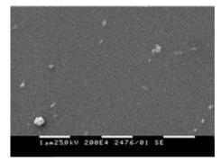
Fig. 5. SEM image of vacuum deposited  $ZnPc:C_{60}$  composite film. Thickness:147.0±0.4 nm.
