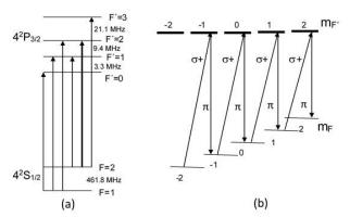
**Fig. 2.** (a) Energy level diagram of the  $4^2S_{1/2} \rightarrow 4^2P_{3/2}$  transitions (D<sub>2</sub> line) of <sup>39</sup>K. (b) Simplified energy level diagram. Zeeman splitting of the F = 2 level is only shown because the F' = 2 level splitting is much less than its spectral width.
