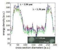
Fig. 8. The 2D computer processing graphs of two spots -at 1.06 and 1.36  $\mu$ m. The spots (in the inset) are marked on the blackened tracing paper A3x type
