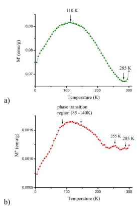
**Fig. 4.** Temperature dependence of the *ac* differential magnetization of Ba<sub>0.5</sub>Sr<sub>1.5</sub>Zn<sub>2</sub>Al<sub>0.08</sub>Fe<sub>11.92</sub>O<sub>22</sub> in an *ac* magnetic field with amplitude 10 Oe and frequency 1 kHz: a) M'(T) – the real part of the differential magnetization; b) M''(T) – the imaginary part of the differential magnetization.
