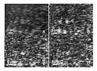
**Fig. 4.** A – a digital hologram of TGS monocrystal, doped with 4% Yb in the solution of growth; B – reconstruction of the intensity of hologram 4A on the surface of the sample, C - reconstruction of the intensity of the hologram 4A at 1  $\mu$ m depth inside the TGS sample and D - reconstruction of the intensity of the hologram 4A at 2  $\mu$ m depth inside the TGS sample.
