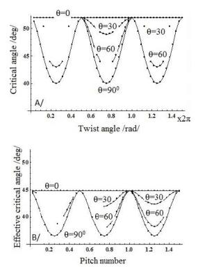
**Fig. 4**. a) Critical angle as a function of twist angle for different tilt angles for nematic layer; b) Effective critical angles as a function of pitch number for different tilt angles for cholesteric layer.
