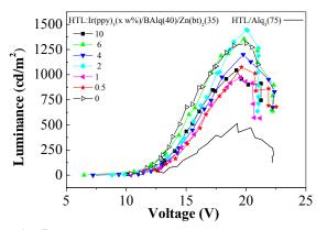
**Fig. 5.** Electroluminescence – voltage characteristics of devicesHTL:Ir(ppy)<sub>3</sub> (x wt.%)/BAlq(40nm)/Zn(bt)<sub>2</sub> (35nm) and HTL/Aq<sub>3</sub>(75nm).
