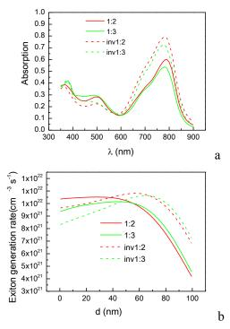
**Fig. 5.** Comparison of calculated optical absorption profiles for devices with standard and inverted structure. The thicknesses of buffer layers  $ZrO_2$  and  $MoO_3$  were set to 20 nm. a) Fraction of incident light absorbed in 100 nm thick  $Sq1/PC_{61}MB$  active layer in dependence of
