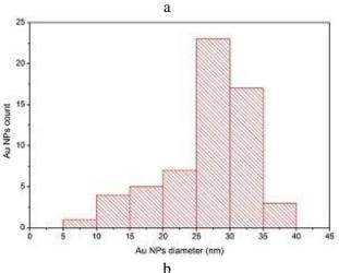
**Fig. 3.** a)FTEM image with 40 000 times magnification of the sample synthesized using citrate method; b) Histogram showing size distribution of 60 gold nanoparticles observed in Fig. 3a.
