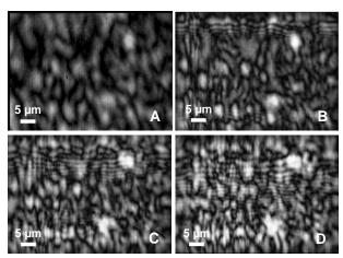
**Fig. 2.** A – a digital hologram of TGS monocrystal, doped with 1% Yb in the solution of growth; B – reconstruction of the intensity of hologram 2A on the surface of the sample, C - reconstruction of the intensity of the hologram 2A at 1  $\mu$ m depth inside the TGS sample and D - reconstruction of the intensity of the hologram 2A at 2  $\mu$ m depth inside the TGS sample.
