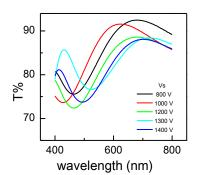
**Fig. 9.** Transmittance spectra of 180 nm thick ITO films, deposited at indicated V<sub>s</sub>.
