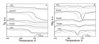
**Fig 4.** TG (a) and DTG (b) data for the samples prepared with CTAB template (solid line) and without (dash line).
