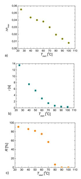
**Fig. 4.** Recording temperature dependences of (a) the maximal induced birefringence, (b) response time, and (c) parameter *R*.
