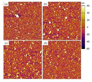
Fig. 2. AFM pictures (10 μm x 10 μm) of the surface of ZnO films deposited on Si-substrate by the electrospray method at applied voltage of 9.5 kV (a), 11 kV (b), 12.5 kV (c) and 13.5 kV (d) and an emitter-to-collector distance of 4 cm (a, b) and 7 cm (c, d).
