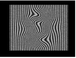
Fig. 2. Computer generated fringe pattern, corrupted with noise.
