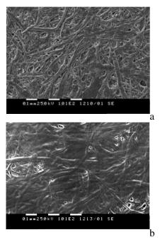
Fig. 4. SEM micrographs of the surface morphology of non-impregnated (a) and PET impregnated paper (b).
