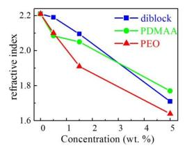
**Fig. 5.** Template concentration dependence of refractive index of porous Nb<sub>2</sub>O<sub>5</sub> films prepared with denoted polymers as templates and annealed at 320 °C for 30 min.
