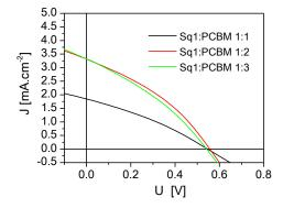
**Fig. 3.** J-V curves for conventional BHJ cells at different weight ratio of the Sq1/PC<sub>61</sub>MB active layers.
