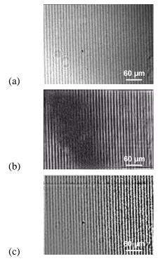
**Fig. 2.** Images of diffraction grating with spatial frequency of 100 lines/mm recorded in Bayfol HX200 photopolymer: a) a digital hologram; b) reconstructed intensity on the surface of the photopolymer layer; c)
