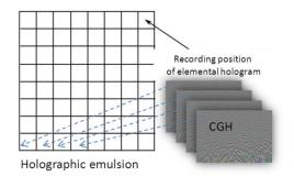
**Fig. 1.** Printing a volume reflection hologram as a collection of elemental holograms recorded from a set of CGHs.
