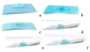
**Fig. 7.** Digital images of the front view of: nonimpregnated paper (a-c); PET impregnated paper (d-f); at the beginning of testing (a, d); in the middle(b, e); at the end (c, f).
