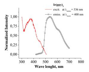
Fig. 2. Excitation (at  $\lambda_{emiss.} = 536$  nm) and photoluminescence emission (at  $\lambda_{excit.} = 536$  nm) spectra of Ir(ppy)<sub>3</sub> CH<sub>2</sub>Cl<sub>2</sub> solution.
