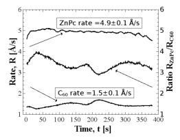
Fig. 2. Typical rates in the co-deposition process for preparation  $ZnPc:C_{60}$  composite as an active BHJ layer in organic solar cell. Right ordinate presents the  $R_{ZnPc}$  / $R_{C60}$  ratio, calculated during the deposition process.
