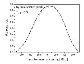
Fig. 5. Double scan: laser frequency slow detuning across the  $D_2$  line and magnetic field faster modulation around B = 0.
