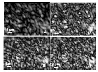
**Fig. 3.** A – a digital hologram of TGS monocrystal, doped with 1% Yb in the solution of growth; B – reconstruction of the intensity of hologram 3A on the surface of the sample, C - reconstruction of the intensity of the hologram 3A at 1  $\mu$ m depth inside the TGS sample and D - reconstruction of the intensity of the hologram 3A at 2  $\mu$ m depth inside the TGS sample.
