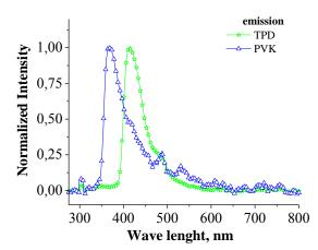
**Fig. 3.** Photoluminescence emission spectra of PVK and TPD in CH<sub>2</sub>Cl<sub>2</sub> solution taken under excitation with tungsten halogen white light sources (LS-1, Ocean Optics Inc.).
