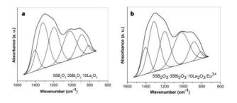
Fig. 3. Deconvoluted IR spectra of: (a)  $55B_2O_3 \cdot 35Bi_2O_3 \cdot 10La_2O_3$  and (b)  $55B_2O_3 \cdot 35Bi_2O_3 \cdot 10La_2O_3$  : Eu<sup>3+</sup> glass samples obtained by melt quenching technique.
