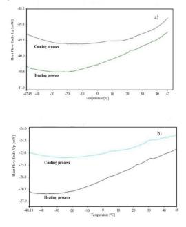
Fig. 3. DSC analysis on as-received TiNb archwires 0.017x0.025 inches<sup>2</sup> (a) and 0.019x 0.025 inches<sup>2</sup> (b)
