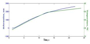
**Fig. 4.** Comparison between the temperature growth and the deformation growth at given point of the deformation field.
