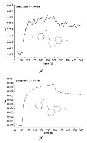
**Fig. 2.** Time dependence of the photoinduced birefringence  $\Delta n$  in Azo-d in case of recording with pump lasers with wavelengths: (a) 355 nm, and (b) 444 nm, respectively.
