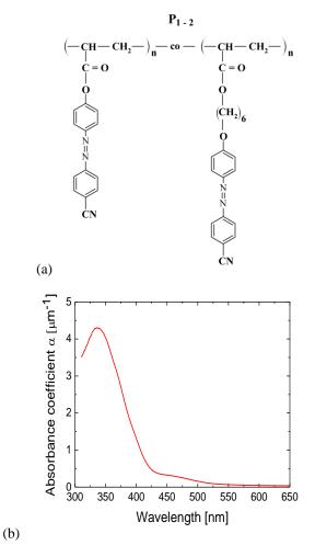
**Fig. 1.** (a) Chemical structure of the azocopolymer P<sub>1-2</sub>; (b) Spectrum of absorbance of P<sub>1-2</sub>.
