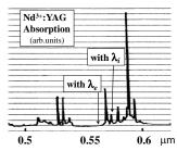
**Fig. 6.** The parts of the absorption spectrum of Nd<sup>3+</sup>-ions in the YAG crystal and the wavelengths of the illuminating laser beams [13].
