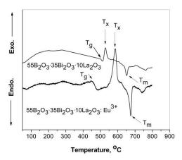
**Fig. 5.** DTA curves of  $55B_2O_3 \cdot 35Bi_2O_3 \cdot 10La_2O_3$  and  $55B_2O_3 \cdot 35Bi_2O_3 \cdot 10La_2O_3 : Eu^{3+}$  glass samples obtained by melt quenching technique.
