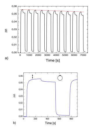
Fig. 3. (a) Ten cycles of inducing and optically deleting linear birefringence; (b) Zoom on the first cycle. The symbols indicate the state of polarization of the laser with  $\lambda = 444$  nm.
