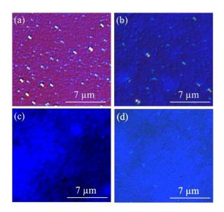
**Fig. 3.** Optical microscopic images of electrosprayed ZnO using applied voltage of 9.5 kV (a,b) and 13.5 kV (c,d), emitter-to-collector distance of 4 cm (a,b) and 7 cm (c,d) before (a, c) and after annealing at 550 °C (b,d).
