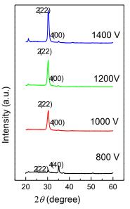
**Fig. 3.** X-ray diffraction patterns of 180 nm thick ITO films, deposited at indicated sputtering voltage.
