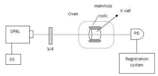
**Fig. 1.** Experimental set-up diagram: DFBL - distributed feedback laser, SG – signal generator,  $\lambda/4$  - quarter-wave plate, PD - Photo-Detector.
