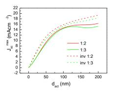
**Fig. 6.** Calculated  $J_{sc}^{max}$  as a function of active layer thickness for the same device structures (as in Fig. 5) under 100 mW cm<sup>-2</sup> AM 1.5G spectral illumination.
