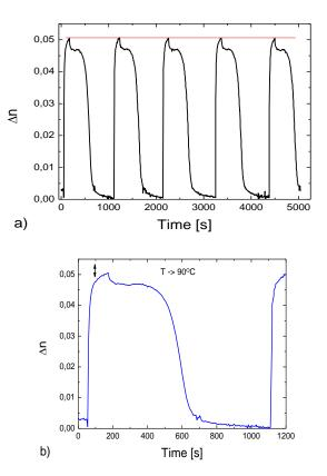
**Fig. 4.** (a) Five cycles of inducing and thermally deleting linear birefringence; (b) Zoom on the first cycle. The arrow indicates the polarization state of the pump laser.
