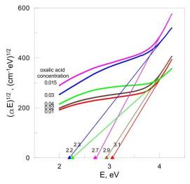
**Fig. 2.** Tauc plots for all oxalic acid concentrations. The tangent straight lines are used to find the optical energy bands shown at the bottom axis.
