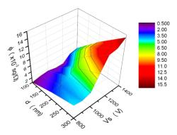
**Fig.10.** Figure of merit as a function of the film thickness and the sputtering voltage.
