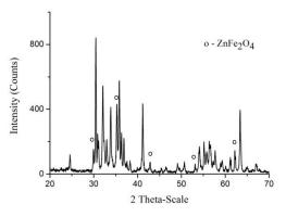
Fig. 1 XRD spectrum of  $Ba_{0.5}Sr_{1.5}Zn_2Al_{0.08}Fe_{11.92}O_{22}$  powder.
