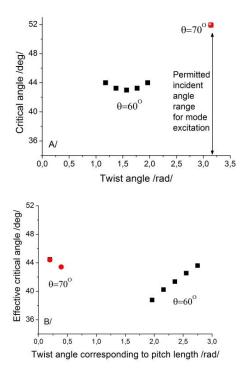
**Fig. 3**. a) Critical angle as a function of twist angle for nematic layer and b) Effective critical angle as a function of twist angle, corresponding to pitch length, for cholesteric layer at different tilt angles.
