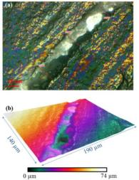
**Fig. 3.** Topography of the representative sample from group MO (50x magnification).
