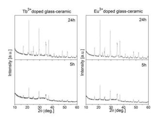
**Fig. 2.** XRD patterns of the samples doped by 0.5 at.% Tb and 0.1 at.% Eu treated at 650°C during 5 and 24h.
