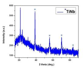
**Fig. 1.** XRD pattern on TiNb archwire 0.019x0.025 inches<sup>2</sup>
