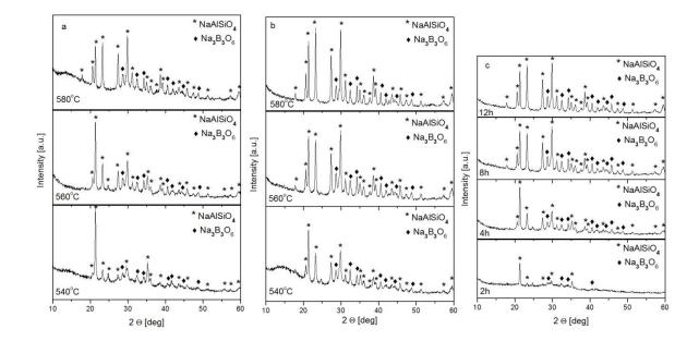
**Fig. 3.** XRD patterns of the glass-ceramic obtained from the glass with composition numbered 7 treated at (a) 540, 560 and 580°C during 4h; (b) 540, 560 and 580°C during 8h; (c) 560°C during 2, 4, 8 and 12h.
