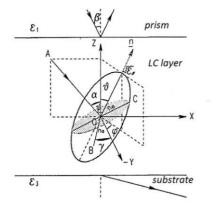
**Fig. 1**. Configuration of the structure and orientation of the principle axes of the local dielectric tensor ellipsoid defined by Euler angles in some chiral molecular layer.
