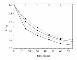
Fig. 5. Photodegradation effect of MO as a function of irradiation time of commercial TiO<sub>2</sub> P25 Degussa ( $\bullet$ ), and mechanochemically synthesized samples ZnS ( $\triangleright$ ), ZnS/TiO<sub>2</sub>-1( $\Box$ ), ZnS/TiO<sub>2</sub>-2 ( $\bullet$ ) and blank experiment ( $\circ$ ).
