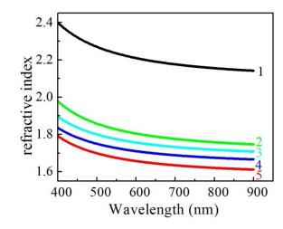
**Fig. 2.** Refractive index as a function of wavelength for Nb<sub>2</sub>O<sub>5</sub> thin films deposited without organic template (curve 1) and with addition of PDMAA (curve 2), PDMAA-*b*-PEO-*b*-PDMAA (curve 3), PDMAA-*b*-PEO (curve 4) and PEO (curve 5) with ratio of template to NbCl<sub>5</sub> equals to 0.23. All films were annealed at 320 °C for 30 min.
