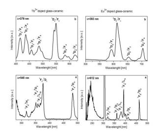
**Fig. 3.** Excitation (a) and emission (b) spectra of the 0.5 at.% Tb doped glass-ceramic sample and 0.1 at.% Eu doped glass-ceramic sample treated at 650°C during 24h. CIE 1931 coordinates for Tb<sup>3+</sup> doped sample x=0.23, y=0.27. CIE 1931 coordinates for Eu<sup>3+</sup> doped sample x=0.45, y=0.29.
