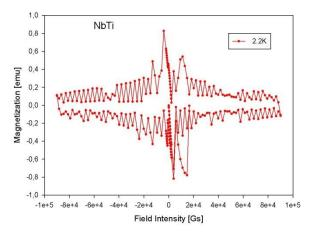
Fig. 5. Magnetic measurements on TiNb archwire  $(0.019 \times 0.025 \text{ inches}^2)$ .
