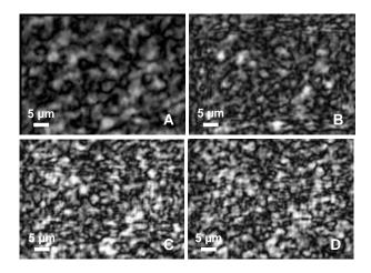
**Fig. 5.** A – a digital hologram of TGS monocrystal, doped with 4% Yb in the solution of growth; B – reconstruction of the intensity of hologram 5A on the surface of the sample, C - reconstruction of the intensity of the hologram 5A at 1  $\mu$ m depth inside the TGS sample and D - reconstruction of the intensity of the hologram 5A at 2  $\mu$ m depth inside the TGS sample.
