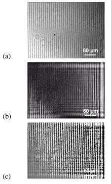
**Fig. 4.** Images of a diffraction grating with spatial frequency of 100 lines/mm recorded in Bayfol HX Photopolymer: a) a digital hologram; b) reconstructed
