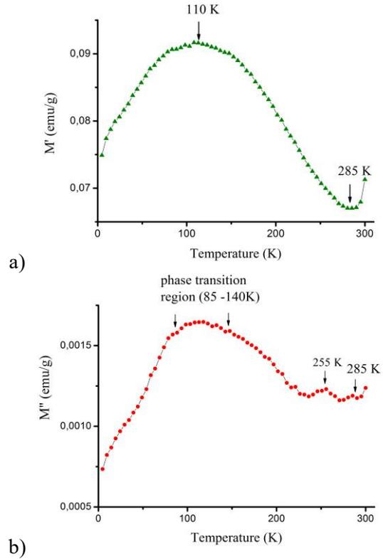
**Fig. 4.** Temperature dependence of the  $ac$  differential magnetization of  $Ba_{0.5}Sr_{1.5}Zn_2Al_{0.08}Fe_{11.92}O_{22}$  in an  $ac$  magnetic field with amplitude 10 Oe and frequency 1 kHz: a)  $M'(T)$  – the real part of the differential magnetization; b)  $M''(T)$  – the imaginary part of the differential magnetization.
