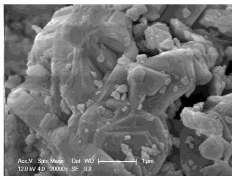
**Fig. 2.** SEM image of  $Ba_{0.5}Sr_{1.5}Zn_2Al_{0.08}Fe_{11.92}O_{22}$  powder.
