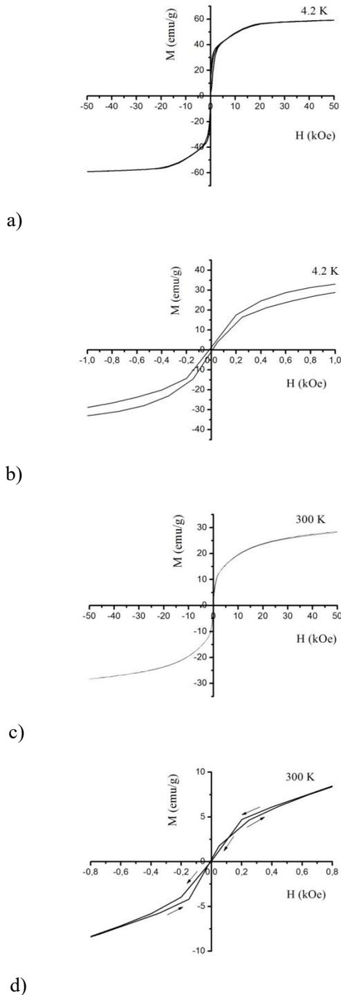
**Fig. 3.** Magnetization measurements of  $Ba_{0.5}Sr_{1.5}Zn_2Al_{0.08}Fe_{11.92}O_{22}$  powder at 4.2 K (a) and 300 K (c); (b) and (d) - expanded view of the hysteresis loops in the low magnetic field range at 4.2 K and 300 K, respectively.
