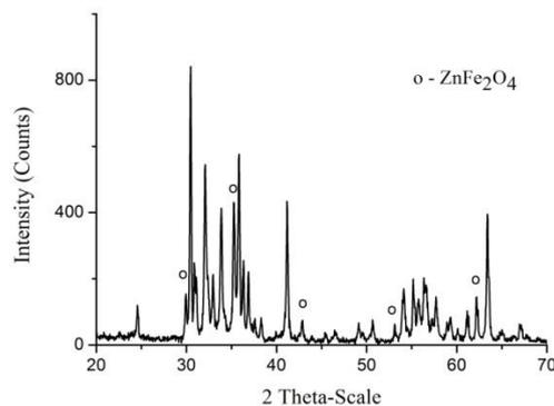
**Fig. 1** XRD spectrum of  $Ba_{0.5}Sr_{1.5}Zn_2Al_{0.08}Fe_{11.92}O_{22}$  powder.
