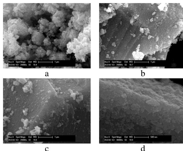
**Fig. 2.** SEM images of BaFe<sub>12</sub>O<sub>19</sub> powders: (a) - YLT1A, (b) - YLT1B, (c, d) - YLT1C.
