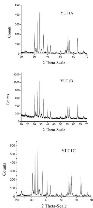
**Fig. 1.** XRD spectra of BaFe<sub>12</sub>O<sub>19</sub> powders: (a) - YLT1A, (b) - YLT1B, (c) - YLT1C.
