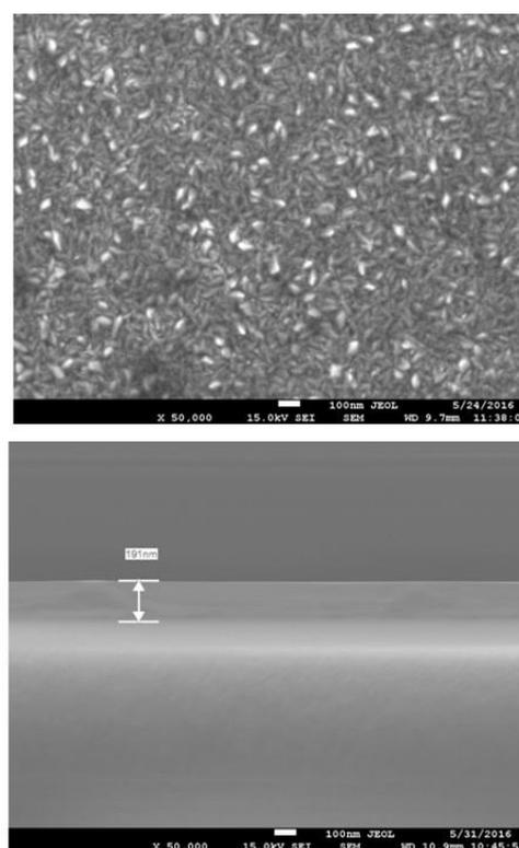
**Fig. 5.** SEM plan view and cross-section of AZO film showing polycrystalline morphology and smooth interface between the film and Si wafer substrate
