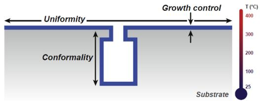
**Fig. 1.** ALD method features: precise growth and thickness control, high conformality/step coverage, good uniformity on large substrates, low substrate temperatures [4].
