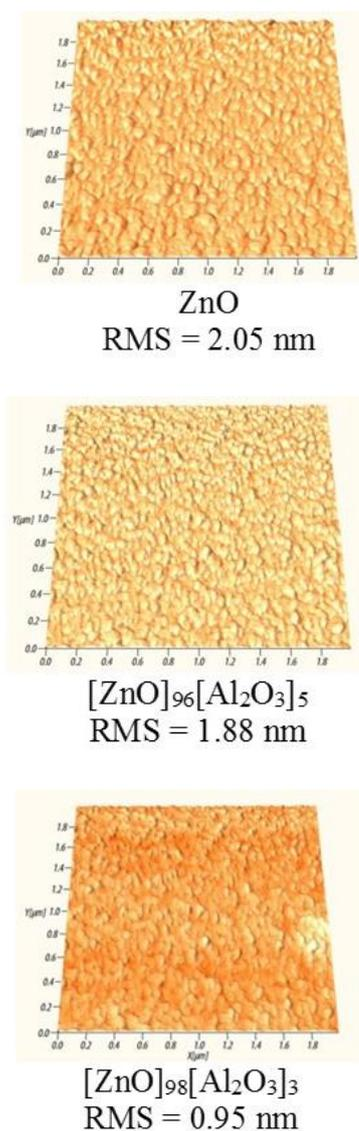
**Fig. 4.** AFM of ZnO and Al-doped ZnO (AZO).
