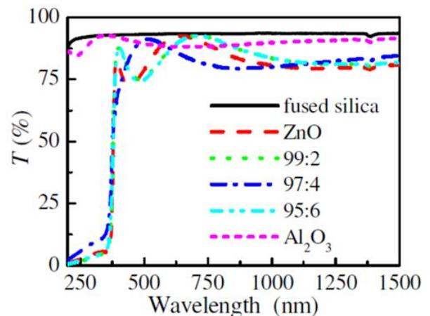
**Fig. 3.** Transmittance spectra of  $\text{Al}_2\text{O}_3$ , ZnO and samples with compositions ZnO:  $\text{Al}_2\text{O}_3$  (cycles ratio shown)
