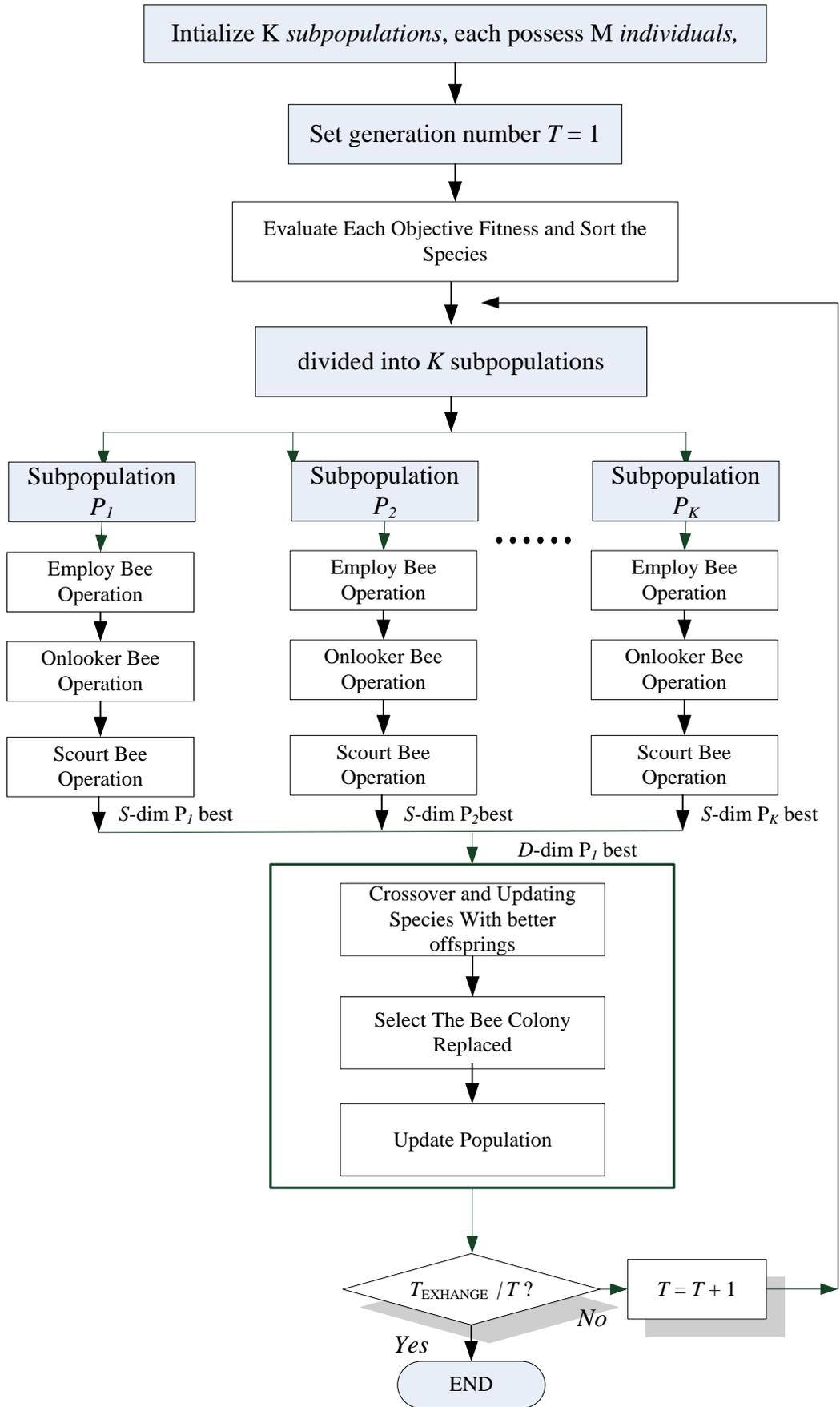
Fig. 2. The flowchart of the proposed artificial bee colony algorithm.
