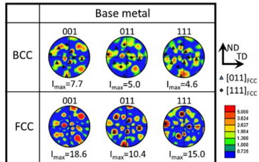
Fig. 4. The diffraction pattern of grain orientation in the same area of the base material.
