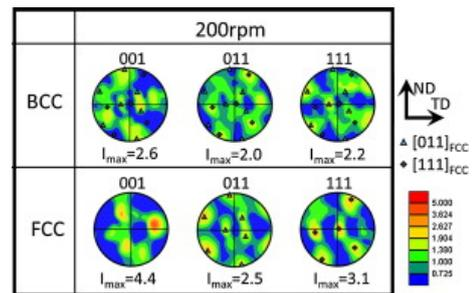
Fig. 7. The orientation of the mixing zone of the 200r/min joint with a rotation speed.
