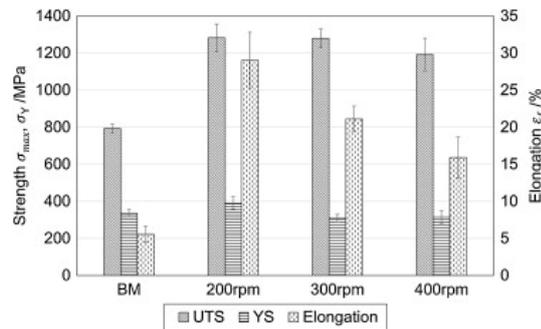
**Fig. 14.** The tensile properties of the base metal and the mixing zone.
