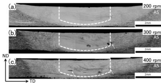
Fig. 5. Optical microscopy: (a) 200r/min (b) 300r/min (c) 400r/min of the joints at different rotation speeds.
