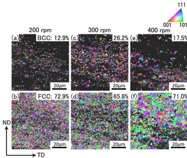
Fig. 6. The crystallization orientation of the joint in the mixing zone. (a,b)200r/min (c,d)300r/min (e,f)400 r/min.
