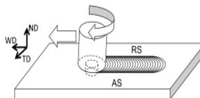
**Fig. 1.** Schematic diagram of friction stir welding.
