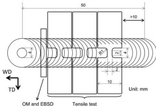
Fig. 2. Geometry and sampling locations of the tensile specimen.
