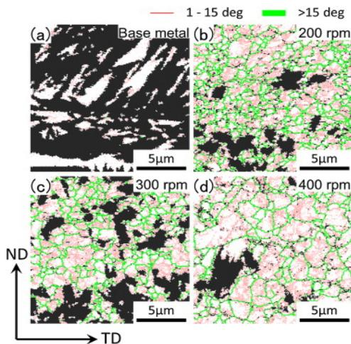
Fig. 10. Grain orientation difference distribution of the base material (a) and stir zone (B, C, d) in the FCC phase.
