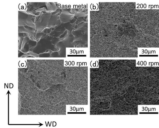
**Fig. 15.** Fracture surface of a and D (c) in room temperature tensile test specimens.
