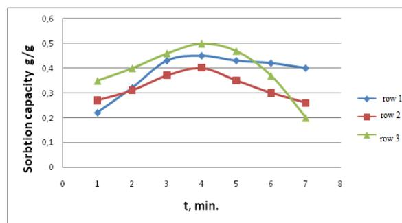
**Fig.2.** Dependence of the sorption capacity of the sorbents on the sorption duration: 1 - rubber foam + carbonizate of sunflower husk (FRCSH- 300) ; 2 - polystyrene foam + carbonizate of rice husk (PFCRH-400) ; 3 - modified rubber foam (MFR-300)
