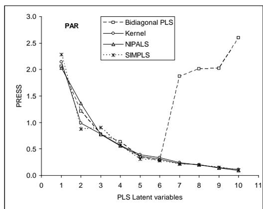
**Fig 3 b)** PRESS-Latent variables plots for different PLS-variants as obtained by cross-validation technique for PAR
