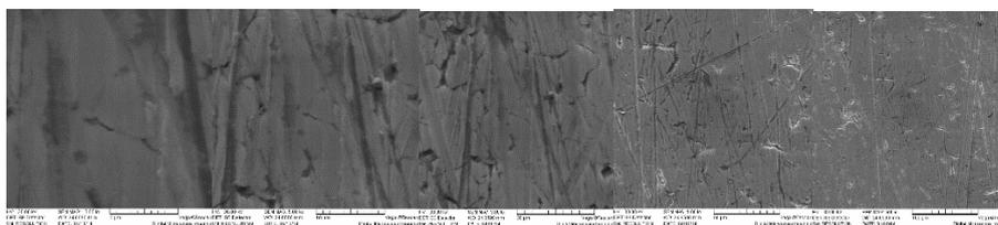
Fig 4-1a. SEM results of specimen before immersed in MDEA+PZ (8:2) blended rich amine solutions
