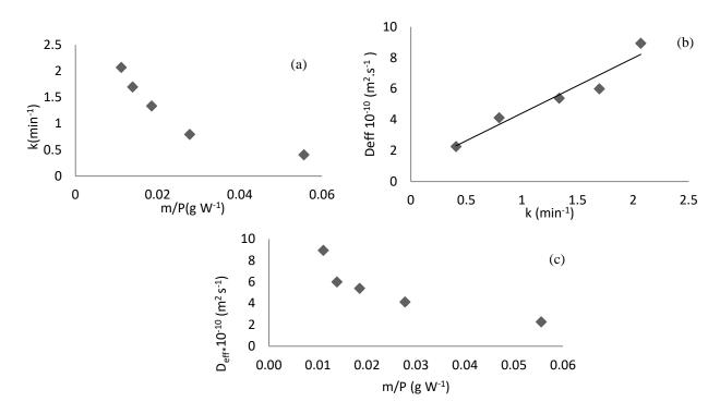
**Fig. 3.** (a) Relationship between the drying rate constant (k) of Page model and the sample mass /power ratio, (b) Relationship between the drying rate constant (k) and the effective moisture diffusivity ( $D_{eff}$ ) for microwave drying of corn husks ( $\blacksquare$  calculated data; - model), (c) Relationship between the effective moisture constant and the sample mass.
