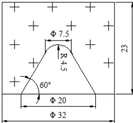
Fig. 2. Structure and size of the horn-shaped booster pellet
