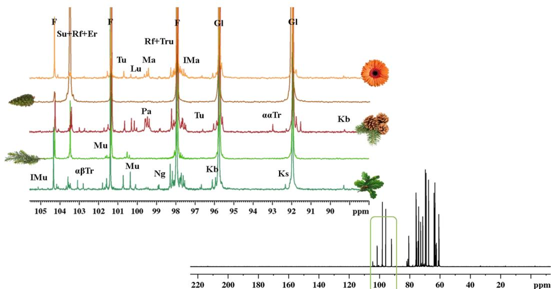
Fig. 2. <sup>13</sup>C NMR spectra of the investigated jams and honeys with expansion of the anomeric sugar region.
