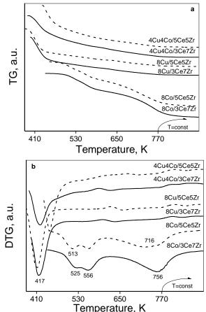
**Fig. 4.** TG (a) and DTG (b) data for the studied Cu and/or Co modifications.
