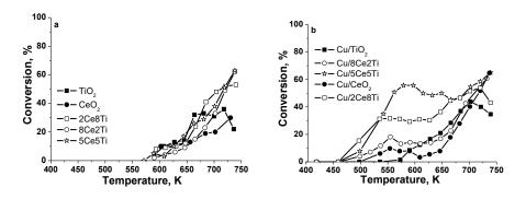
Fig. 6. Mehtanol conversion of CeTi (a) and Cu/CeTi materials (b).
