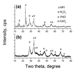
Fig. 1. XRD patterns of: (a) PdO-CeO<sub>2</sub>/ZSM5, (b) PdO-CeO<sub>2</sub>/Al<sub>2</sub>O<sub>3</sub>.
