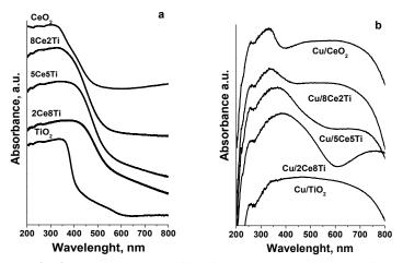
Fig. 2. UV-Vis patterns of CeTi (a) and Cu/CeTi (b) materials
