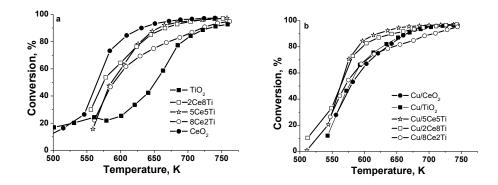
Fig. 5. Ethyl acetate conversion of CeTi (a) and Cu/CeTi (b) materials.
