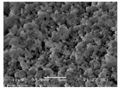
Fig. 2. SEM picture of PdO-CeO<sub>2</sub>/ZSM5 sample.
