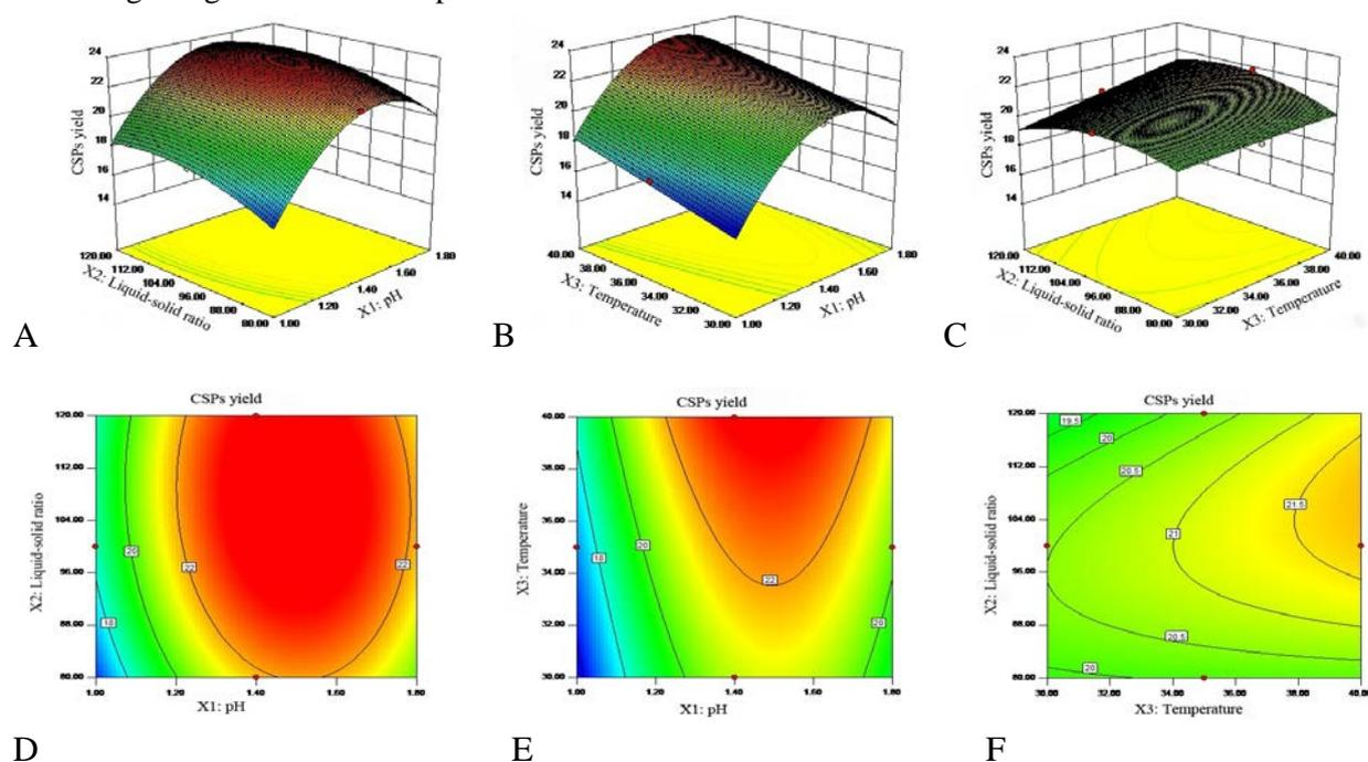
**Fig. 2.** Response surface plots (A, B, and C) and contour plots (D, E, and F) showing the effects of the interaction of proteolysis pH, liquid-solid ratio, and proteolysis temperature on the response of CSPs yield.
