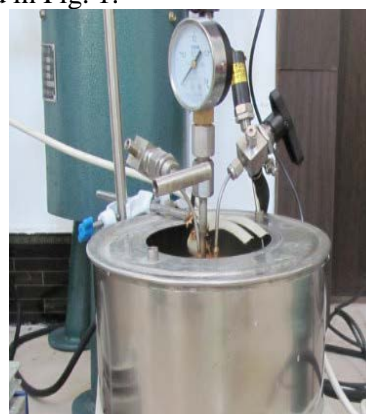
Fig. 1. Experimental setup of the safety chemistry of the ClO 2 oxidation of the oil/water transition layer
