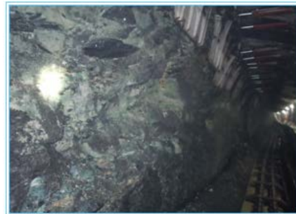
(a) Section of working face passing through cutting layer
