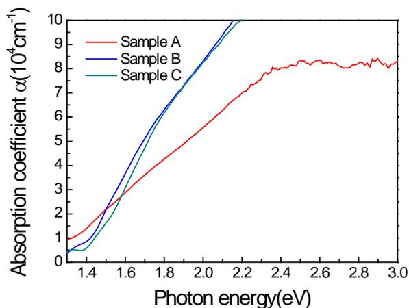
**Fig. 3.** Absorption coefficients of the CZTS films, the letters correspond to their sputtering pressure, A 0.5Pa, B 0.3Pa, C 0.2Pa.
