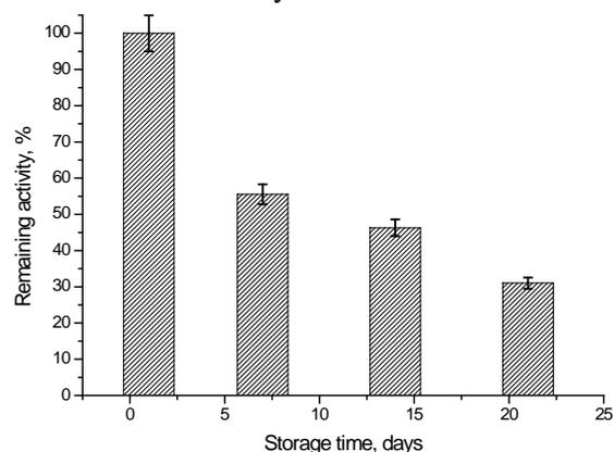
**Fig. 7.** Remaining activity of the laccase electrode as a function of storage time (days). The remaining activity was normalized *vs.* the response of the freshly prepared electrode.
