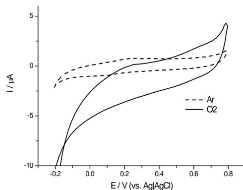
**Fig. 3.** CVs of a laccase (*Trametes pubescens*) electrode in de-aerated with Ar (dashed) and oxygenated (solid) 0.05 M citrate buffer, containing 0.1 M NaClO<sub>4</sub>, pH = 4.5;  $v = 10 \text{ mV s}^{-1}$ ; 25 °C.
