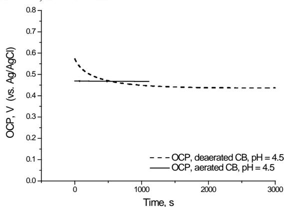
**Fig. 6.** Open circuit potential of the laccase electrode in oxygenated buffer solution (0.05 M citrate buffer + 0.1 M NaClO<sub>4</sub>), pH 4.5; partly deaerated buffer (dashed line); continuously aerated buffer (solid line).
