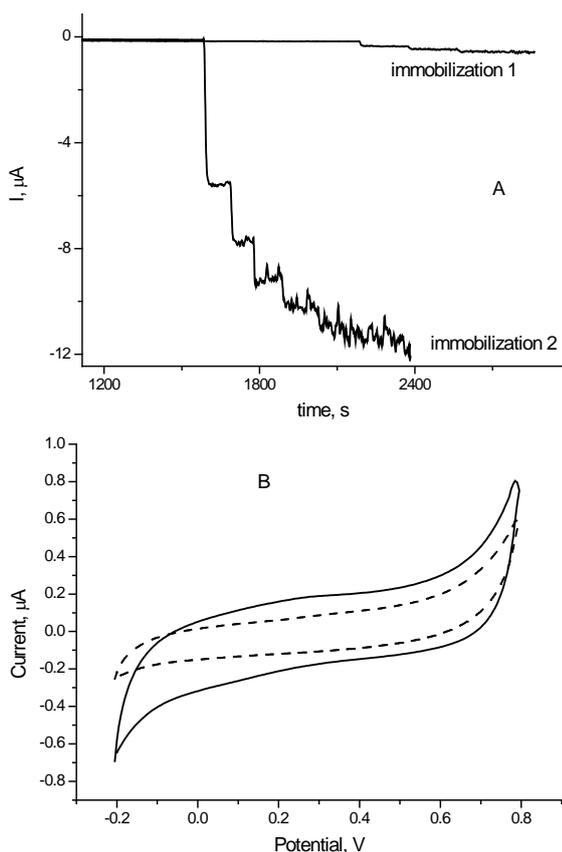
**Fig. 5.** A) Chronoamperometric record of the laccase electrode response to ABTS in presence of oxygen. Laccase enzyme immobilized covalently on gold (curve 1) and gold-thin film -modified glassy carbon (curve 2); pH = 4.5; E = -100 mV
