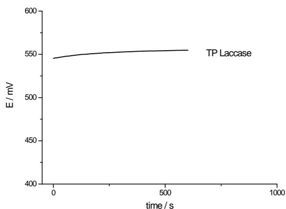
**Fig. 4.** Open circuit potential of the laccase electrode under oxygenated conditions (0.05 M citrate buffer + 0.1 M NaClO<sub>4</sub>), pH 4.5.
