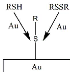
**Scheme 1.** Surface functionalization of gold surface with sulfur-containing organic compounds – thiols or disulfides.
