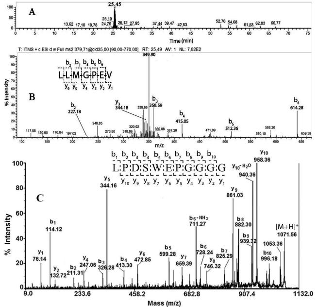
**Figure 1.** A) Extracted chromatogram, B)  $MS^2$  fragmentation of LLMGPEV peptide with m/z 379.17 [M+2H]<sup>2+</sup>, C) MALDI-MS spectrum (positive ion mode) of the peptide at m/z 1071.56[M+H]<sup>+</sup>. Standard peptide solution was used to calibrate the mass scale of the AutoflexTM III, High Performance MALDI-TOF & TOF/TOF Systems (Bruker Daltonics).
