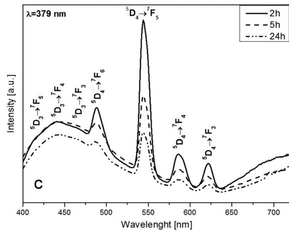
**Fig. 4.** (a) Excitation spectrum of  $Tb^{3+}$  doped glass-ceramic sample treated at 630 °C 2 h; (b) Emission spectra of the  $Tb^{3+}$  doped glass-ceramic samples thermal treated at 580 °C 2, 5 and 24 h; (c) Emission spectra of the  $Tb^{3+}$  doped glass-ceramic samples thermal treated at 630 °C 2, 5 and 24 h.
