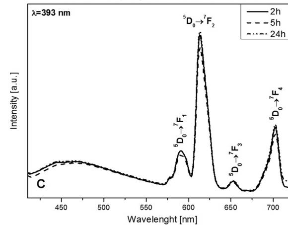
**Fig. 5.** (a) Excitation spectrum of  $Eu^{3+}$  doped glass-ceramic sample treated at 630 °C 2 h; (b) Emission spectra of the  $Eu^{3+}$  doped glass-ceramic samples thermal treated at 580 °C 2, 5 and 24 h; (c) Emission spectra of the  $Eu^{3+}$  doped glass-ceramic samples thermal treated at 630 °C 2, 5 and 24 h.
