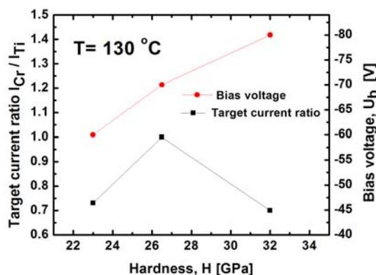
**Fig.4.** Influence of target current ratio I<sub>Cr</sub>/I<sub>Ti</sub> and bias voltage on the nanohardness of the multilayer CrN/TiN coatings
