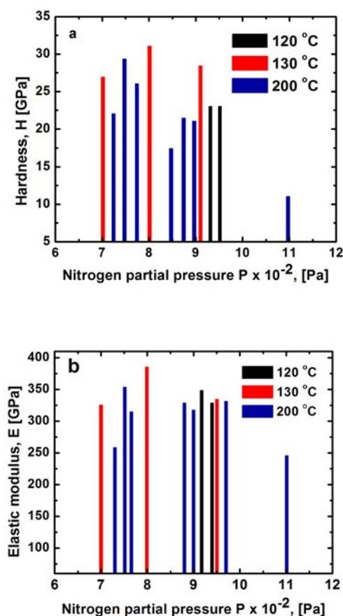
**Fig.3.** Dependence of the nanohardness (a) and elastic modulus (b) of the CrN/TiN coatings on the N<sub>2</sub> partial pressure at different temperatures
