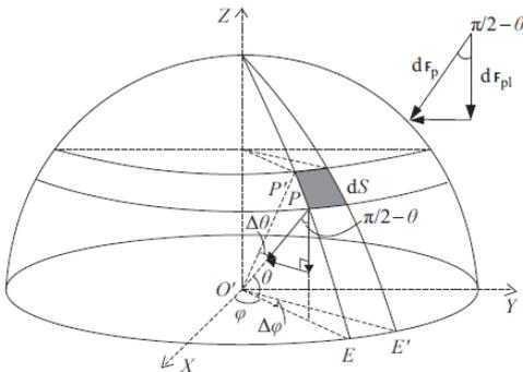
Fig.1. Schematic diagram of force element on the head of capsule
