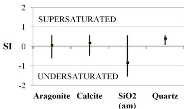
Fig.5. Saturation Index values for thermal waters relative to the major forms of CaCO<sub>3</sub> and SiO<sub>2</sub>
