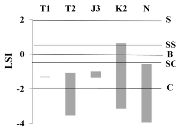
**Fig.3.** Range of variation of LSI values in different age rocks and their comparison with the suggested by Carrier indications [13] (C - Serious corrosion, SC - Balanced but pitting corrosion possible; SS - Slightly scaling and corrosive; S - Scale forming but not corrosive)
