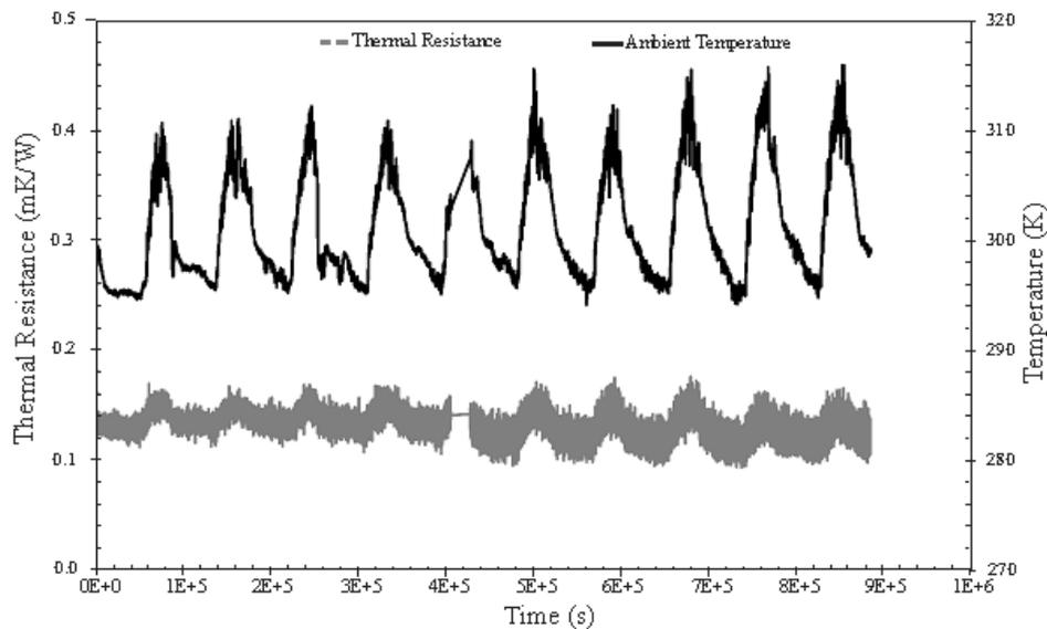
**Fig.9.** Energy pile thermal resistance during the TRT
