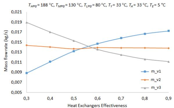
**Fig.9.** Flow rates variations of water vapor with heat exchangers effectiveness
