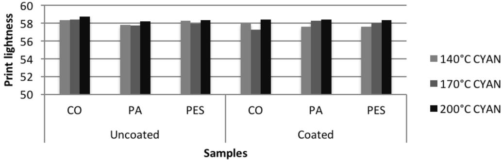
Fig. 1. Print lightness of uncoated and EA coated samples before washing
