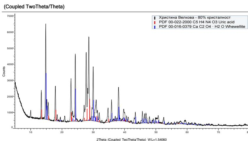
**Figure 7.** XRD pattern of calcium oxalate monohydrate and uric acid
