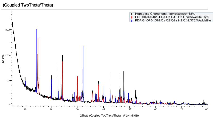
Figure 6. XRD pattern of calcium oxalate monohydrate and dihydrate
