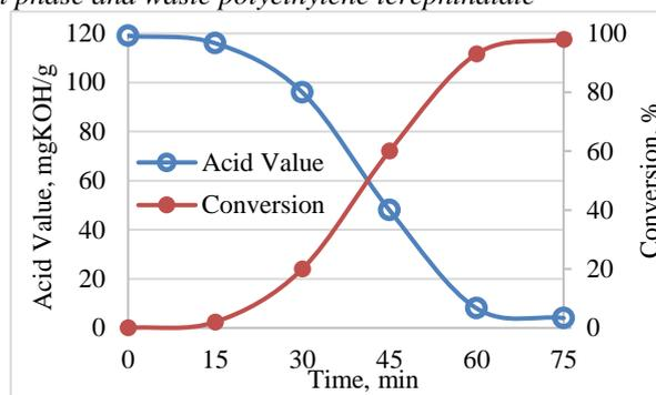
Fig. 1. Change of acid value and conversion during reaction time.
